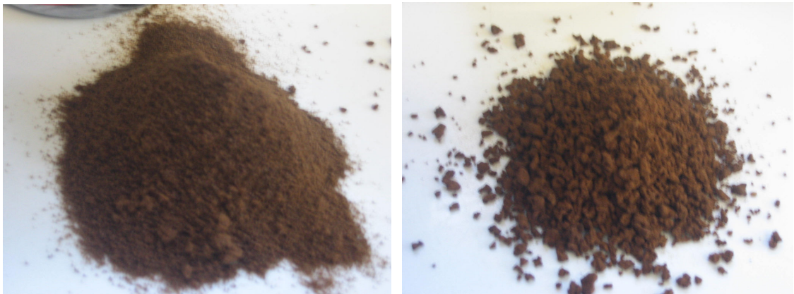
Figure 2: retail coffee: a familiar example of the different product forms obtained by spray drying alone (left) as compared with spray drying followed by granulation (right)
