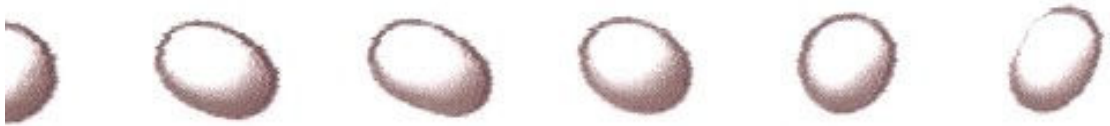
Figure 15: droplet oscillation; droplet stream from breakup of a single jet of 40% solution of glycerol in water, captured under strobe lighting. (ICI - Fanny Briand)
