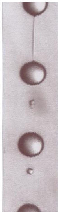
Figure 19: steady satellite droplet formation from a vibrated laminar jet 80% glycerol, 500 \mu m nozzle, 4.3m/s jet velocity, 2.3kHz driving frequency. Fanny Briand, 1999, ICI Wilton.
