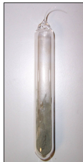
Figure 2-1 Left: high-temperature furnaces used for both synthesis in powder form and crystal growth. Right: typical sealed silica tube containing the reaction mixture.
