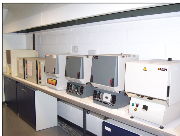
Figure 2-1 Left: high-temperature furnaces used for both synthesis in powder form and crystal growth. Right: typical sealed silica tube containing the reaction mixture.
