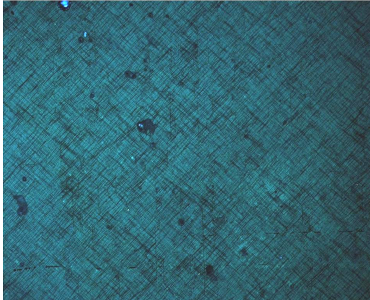
Figure 4.13 UV PL Microscope image of ZnSe. Dark regions indicative of dislocations. Similar cross hatching pattern as seen in figure 4.12
