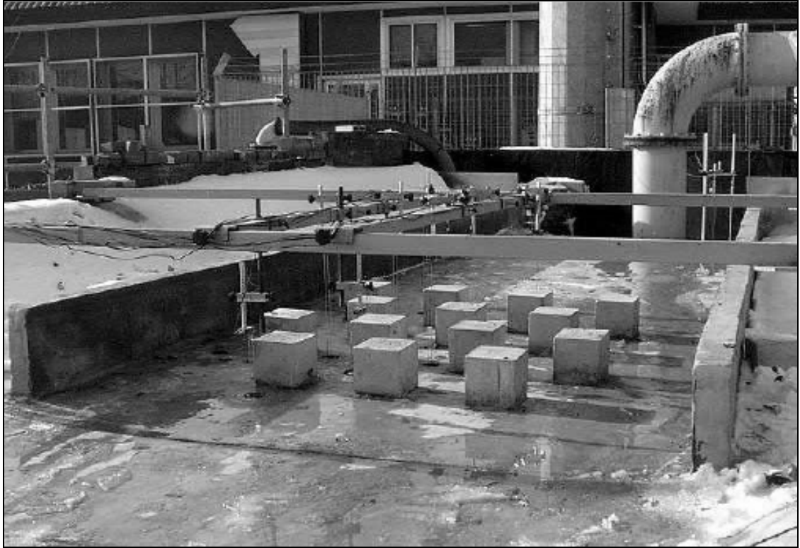
Figure 4.4: Modified topography by placement of two masonry walls (staggered city layout) (Alcrudo et al. 2003)
