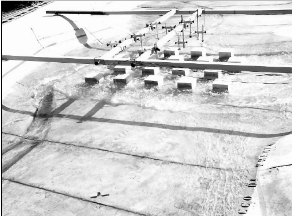
Figure 4.8: A typical run on the original topography with staggered city layout (Alcrudo et al. 2003)
