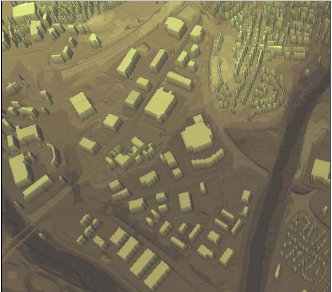
Figure 6.38: Closure view of DEM data created from DTM and MasterMap® data (grid resolution = 3 m)
