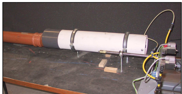
Pneumatic piston installed at base of stack
