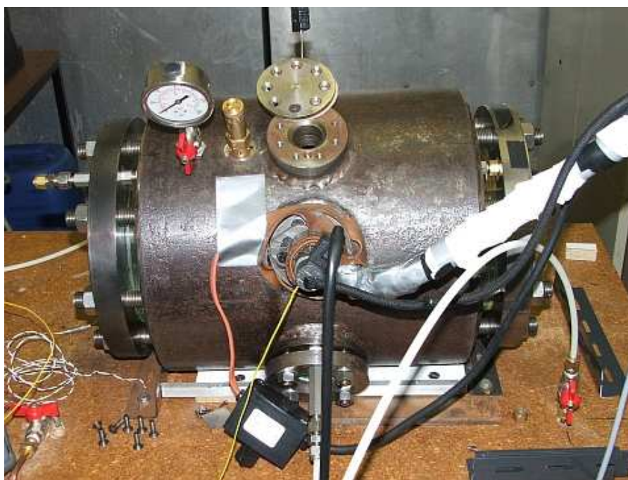
Figure 3.6: The high pressure injection chamber - injection ports and the side window layout.
