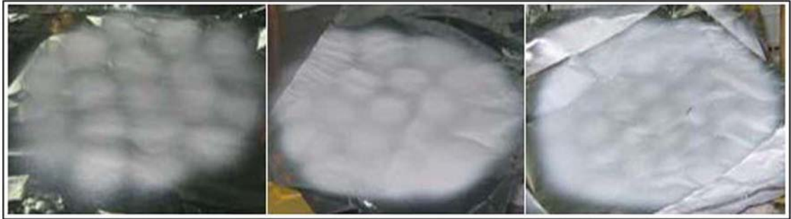
Figure 5.20 , Photographs show collected nanofibre fabric mats electrospun from 19 spinnerets at different inter spinneret distances [71].
