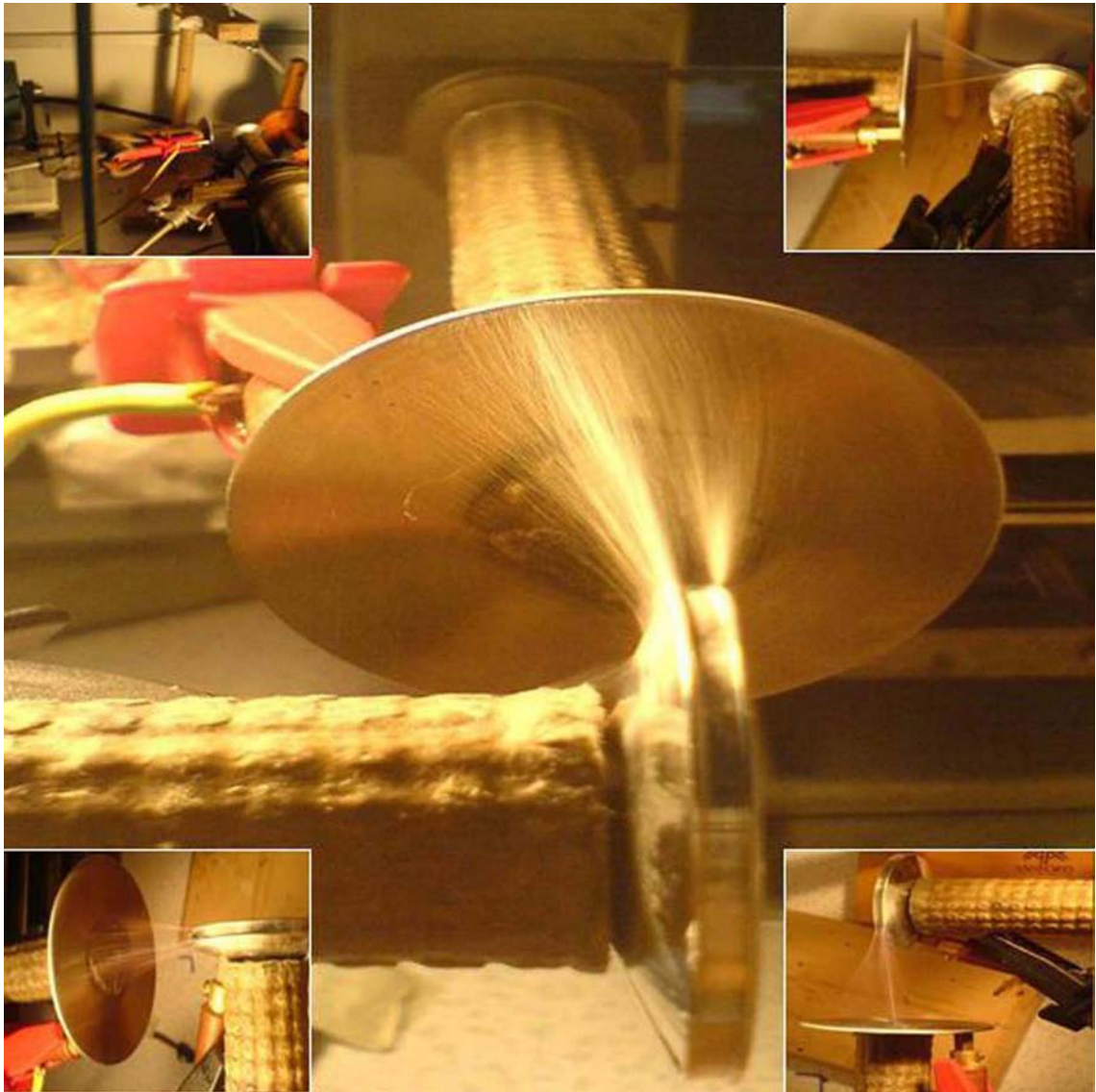
Figure 5.14, A photograph of aligned nylon 6 nanofibres deposited in the gap between the perpendicular twist disk and take up disk for producing continuous core electrospun nano yarn. These nanofibres covered the feeding polyester filament in three dimensional conical architecture. By rotating the twist and take up disks the flying nanofibres deposited helically on the filament to form core electrospun nano yarn.
