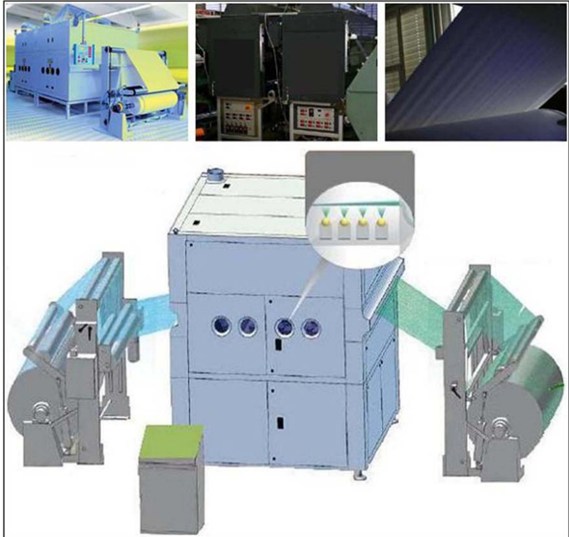
Figure 1.9 , Schematic illustration of the nanospider TM machine produced by Elmarco company [125], (upper left) photograph of nanospider TM machine [125], (upper middle) technical electrospinning set-up with a large scale width presented in TransMIT-Marburg- Germany [117], (upper right) technical textile fabrics coated by electrospun nanofibres [117].
