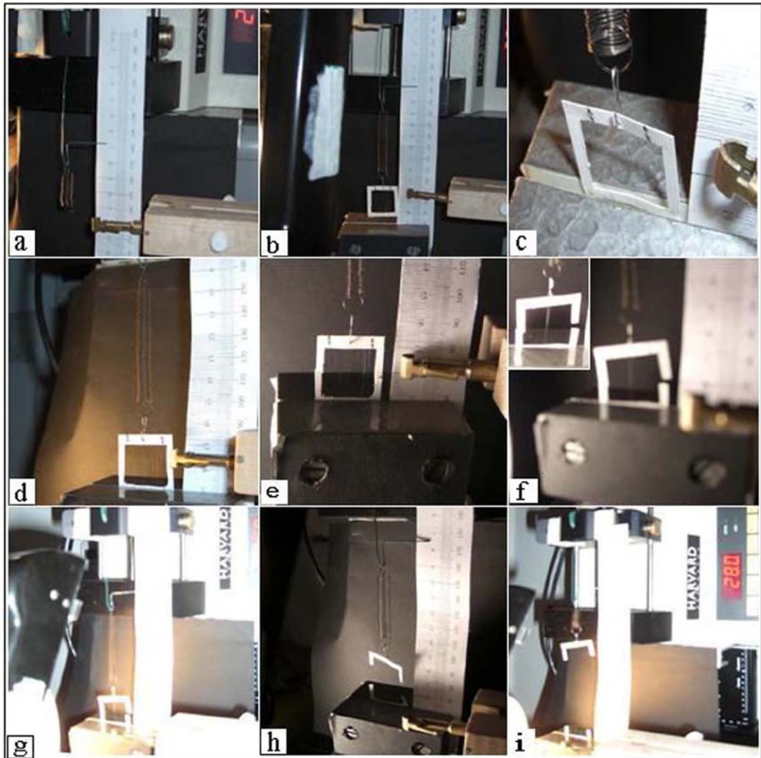
Figure 7.9, Recorded photographs show the tensile test set-up is conducted step by step. (a) Shows the spring ‘transducer’ loaded by its weight only. (b) A cardboard frame containing aligned nanofibres was gripped to the spring, it is clear to see the spring displacement under the frame and nanofibres weight. (c) The cardboard frame was laid on and suspended between the fixed head jaws. (d) The cardboard frame was gripped by the fixed head jaws and its rib was clipped. (e) The cut rib of the cardboard frame (f) Non- required aligned nanofibres were carefully removed and thus a single nanofibre gripped between the fixed head and the spring with a 20 mm gauge length is ready for tensile test. (g) The tensile test process is utilized under a constant loading rate. (h) Tension is still applied on the nanofibre without nanofibre breaking. (i) Breaking ‘failure’ of the tensioned nanofibre has occurred, and the bounce of the upper end of the frame is clear as a result of nanofibre breaking.
