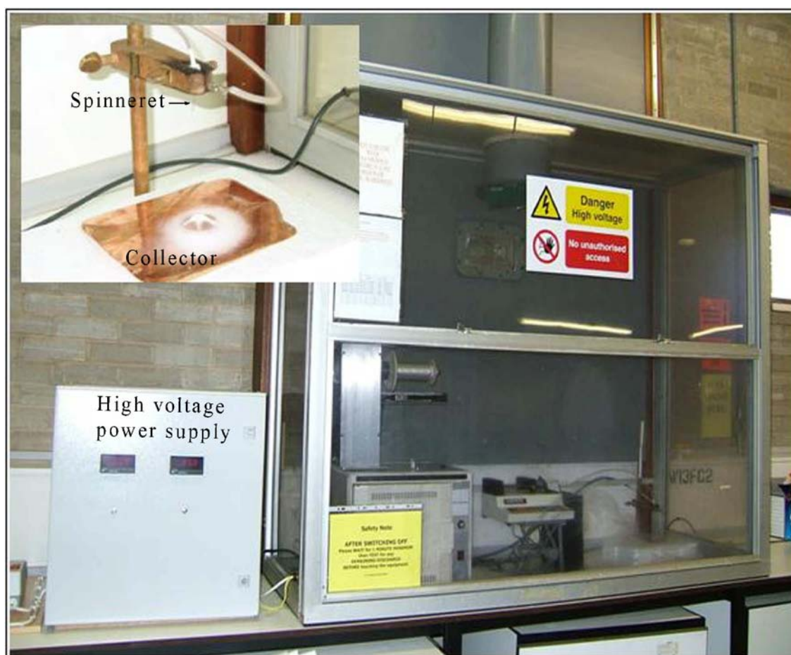
Figure 2.1, A photograph of the experimental electrospinning set-up used in the experiments.
