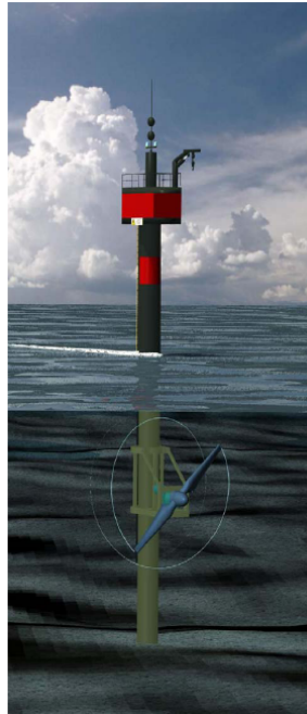
Figure 1.7: The SeaFlow horizontal axis turbine (courtesy of Marine Current Turbines Ltd.)
