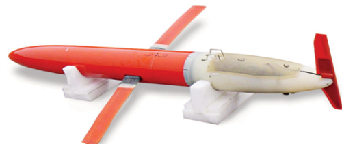
SPRAY Glider AUV (Bluefin) 1
