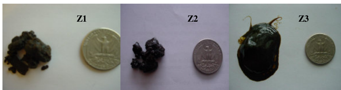
Figure 4.59. Images of different soap deposits from Field Z. Morphologies Z1, Z2 and Z3 indicated in the images.
