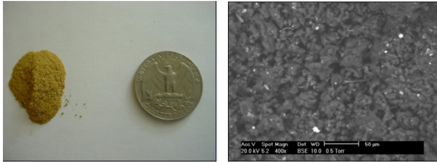
Figure 6.35. Left: Image of clean calcium soap from Field Y soap sample. Right: ESEM image of clean calcium soap from Field Y soap sample.
