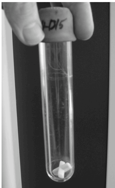
Figure 8.1 A polymerisation tube consisting of a thick-walled test-tube with a septum cap, was used in the preparation of the RAFT copolymers.
