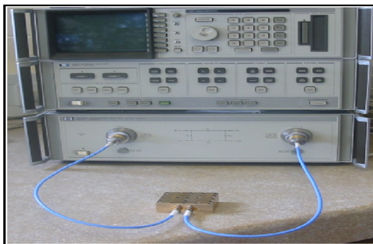
Figure 6-16: Cavity is connected to the HP network analyzer
