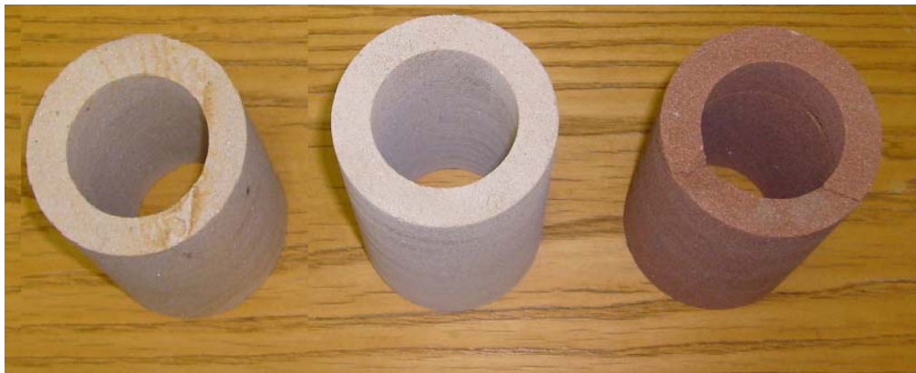
Figure 4.8: 50 mm internal diameter borehole samples made from solid blocks of materials. Left: Clashach sandstone. Center: Doddington sandstone. Right: Locharbriggs sandstone.
