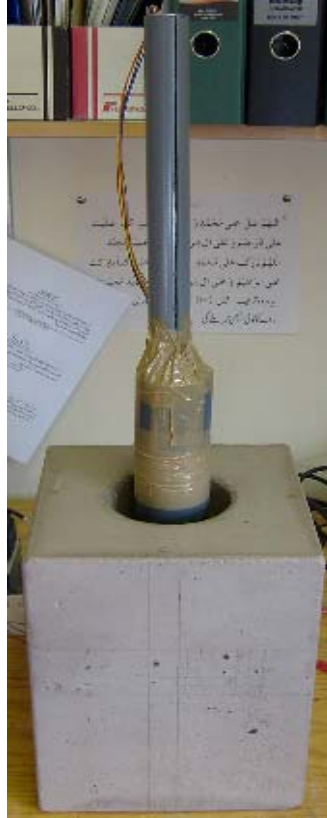
Figure 4.13: A photographic image of the borehole section and the sonde placed in its center.
