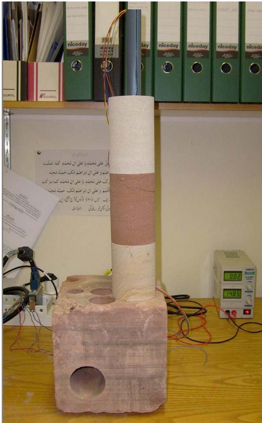
Figure 4.11: Prototype magnetic susceptibility sonde running inside the 50 mm diameter samples (from the top: Doddington, Locharbriggs, and Clashach sandstones) when stacked together in the borehole formation. At the bottom is a solid Locharbriggs block.
