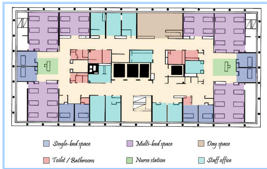
Figure 4.12 - Ward F: Racetrack ward, High Wycombe Hospital in Buckinghamshire, UK. (Original layout: James and Tatton-Brown, 1986)
