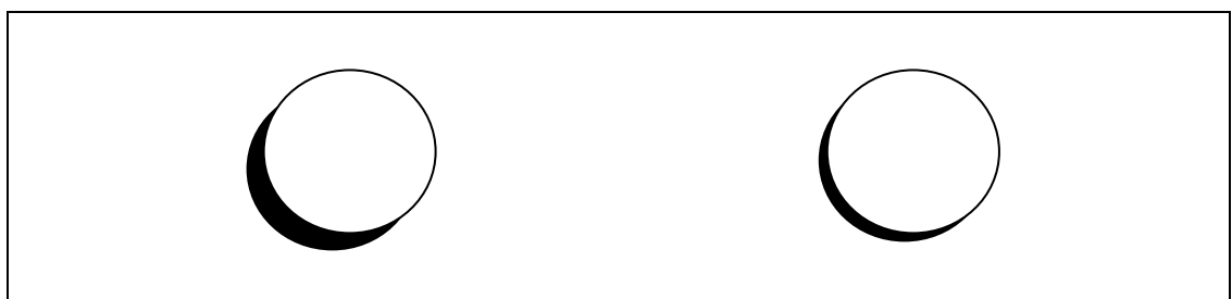
Figure 3-2: Illustration of the bas-relief ambiguity with two cylinders of equal height viewed from above. Because the elevation of the light source is lower for the cylinder on the left, it appears to be taller than the cylinder on the right.
