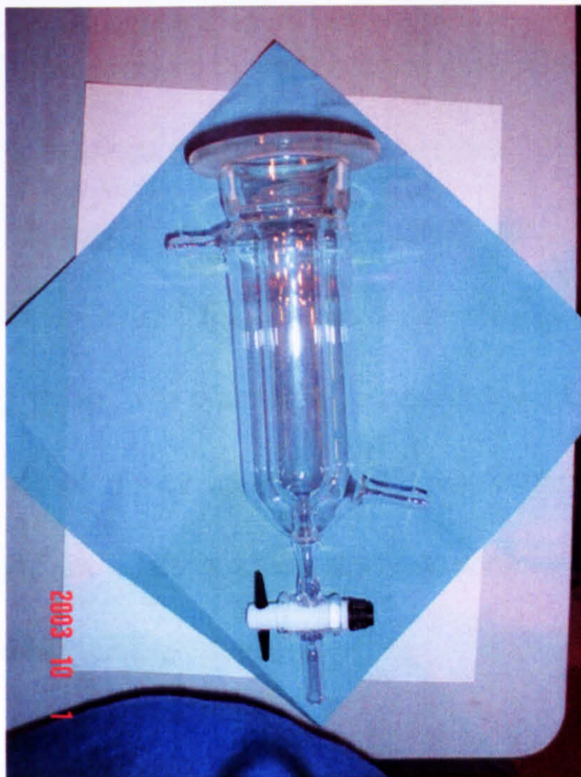
Figure 3.3 Photograph of the jacketed column
