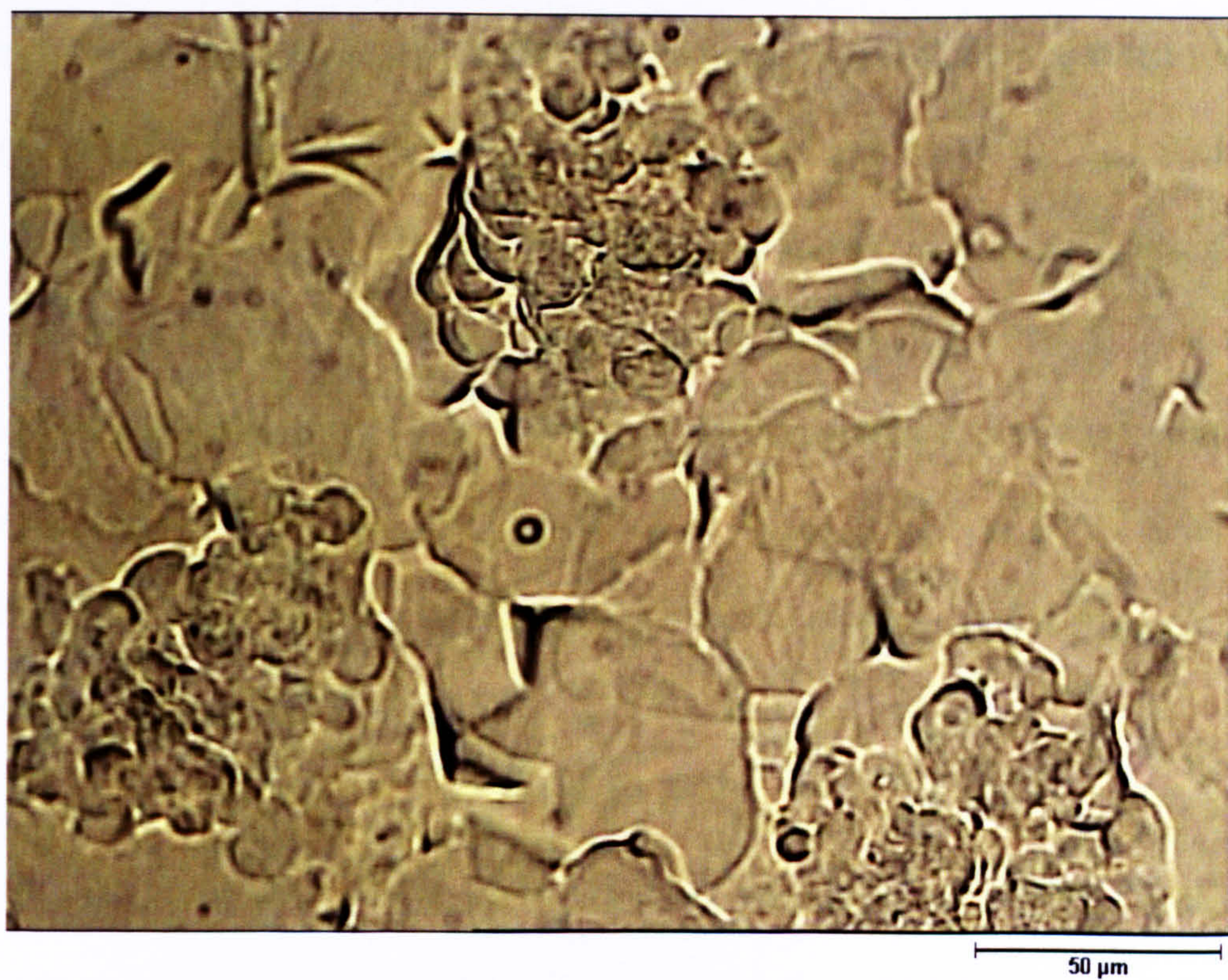
Figure 4.7 Microscopic image of wax crystals from the experiment with oscillation ( x_0 = 15 \text{ mm} , f = 1 \text{ Hz} )
