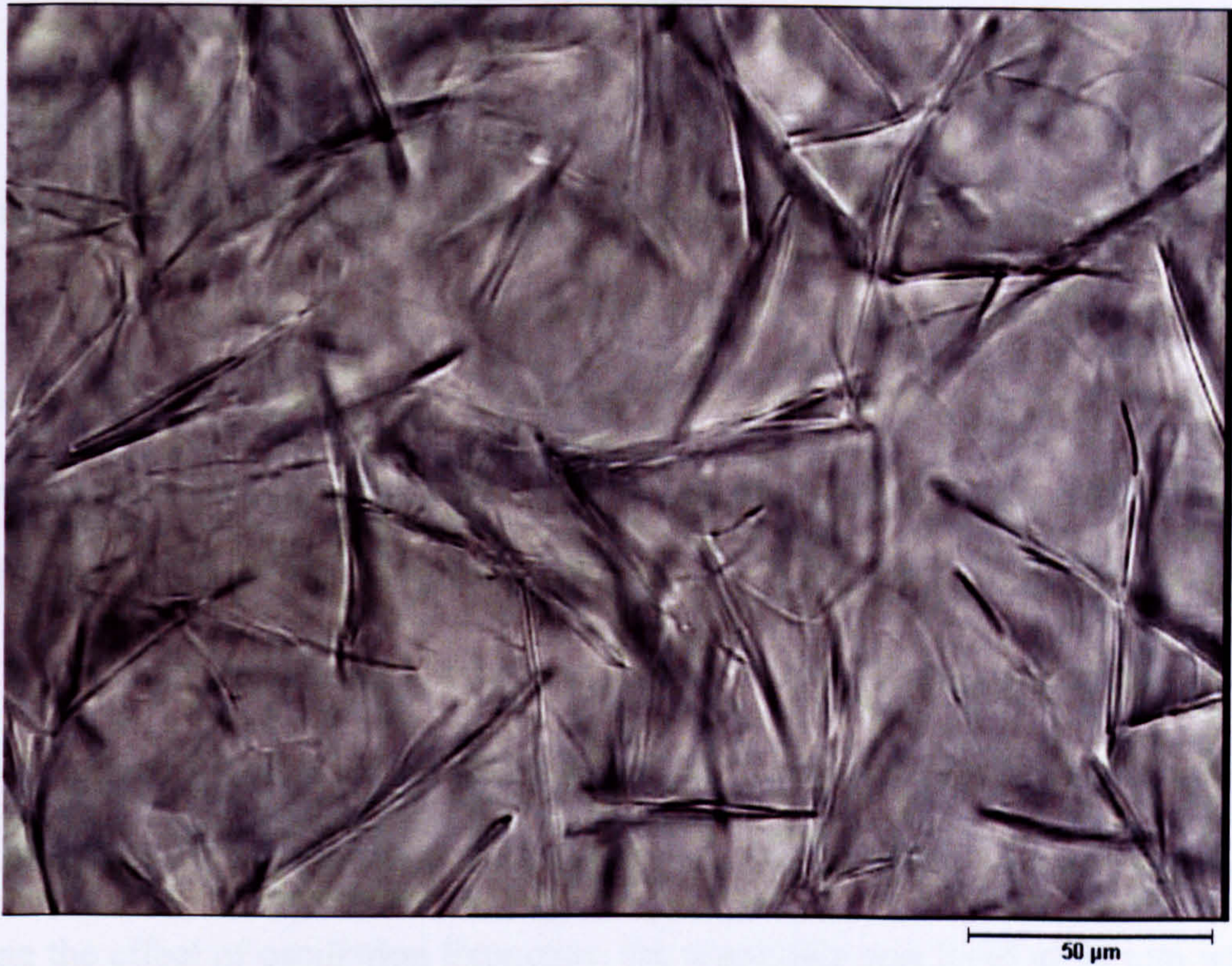
Figure 4.17 Microscopic image of wax crystals from the experiment with no oscillation
