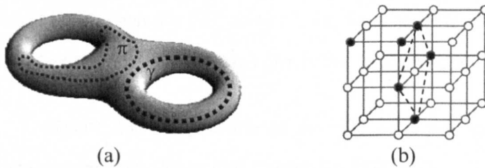
Figure 3-19: Illustration of Definition 3.5: (a) two closed \alpha -paths within a double torus of two tunnels: \pi is shrinkable and \gamma is unshrinkable; (b) the black 18-path cannot be shrunk to a single black voxel, because the central voxel is white, thus revealing a tunnel.
