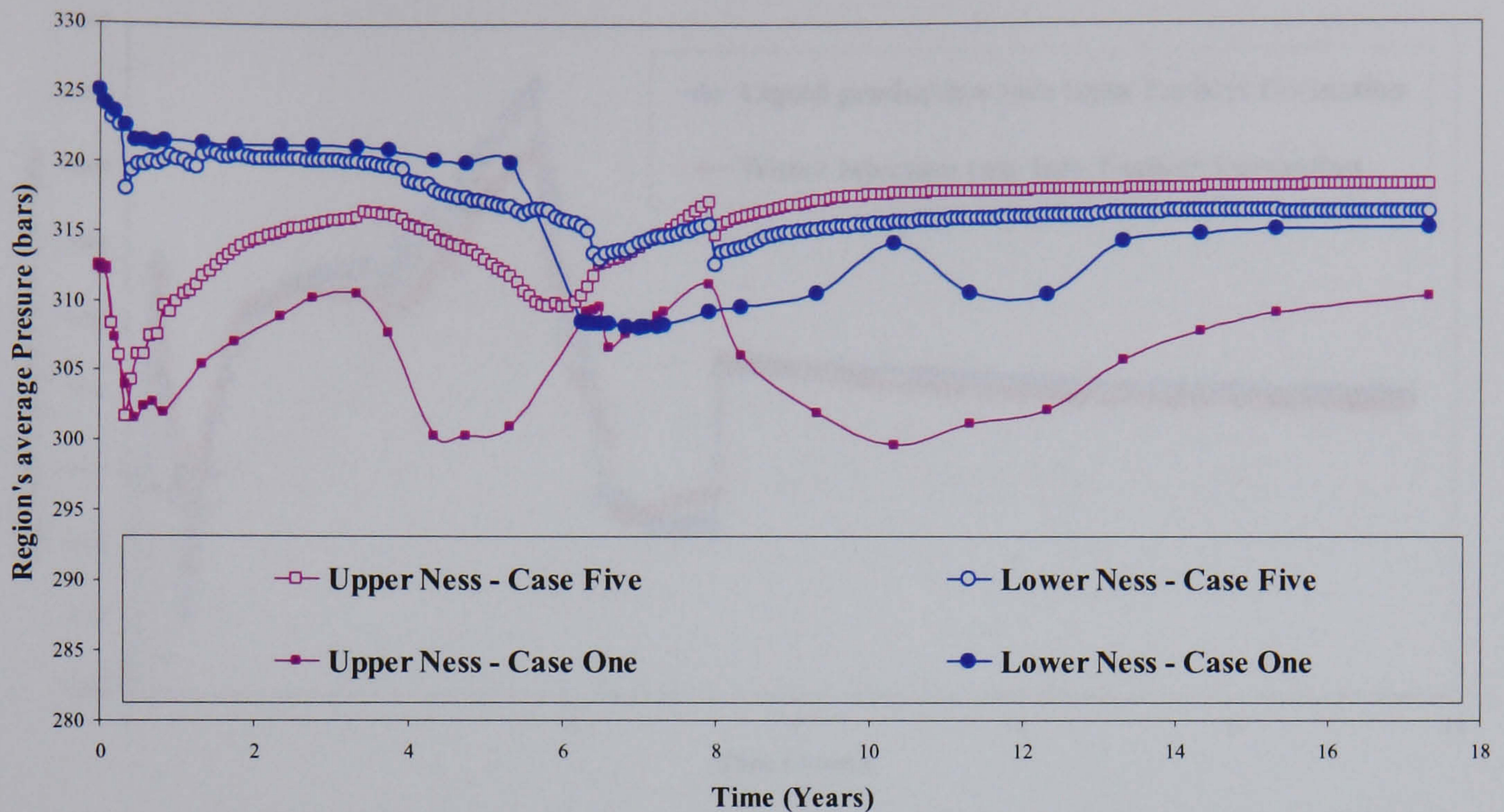
Figure 8.3.1 S-Field Ness Formation pressures for Case One and Case Five Zone voidage replacement was achieved in the model by using the monthly production results from Case Four and estimating the required injection rate based on the volume of liquid produced. This was then used in the smart injection run (Case Five). Figure 8.3.2 shows how effective this technique is at replacing the liquid volume produced from the Tarbert Formation. The same policy was applied to all the zones. The pressure was held reasonably constant, even during the period when the management of the field changed rapidly from 12,000 \text{sm}^3/\text{day} oil to 20,000 \text{sm}^3/\text{day} liquid (year 5). This improved reservoir management scheme not only improves Ness recovery by implementing a full water drive, but also delays the water break through; helping the field to stay on production plateau for longer (Figure 8.3.3). The cumulative total oil production is also increased (Figure 8.3.4). Table 8.1 shows how the combination of intelligent producers and injectors produces the highest oil recovery.
