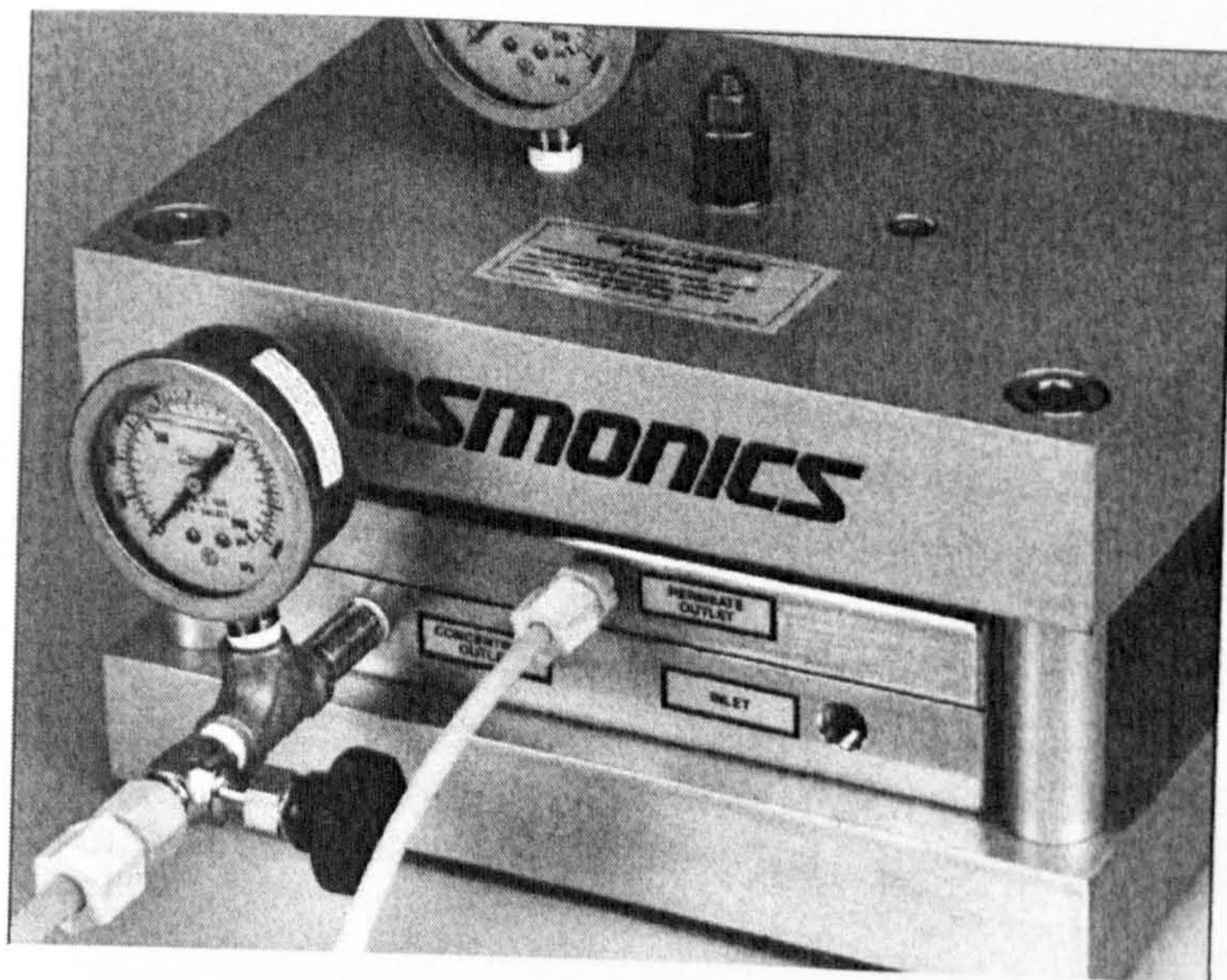
Figure 7. Assembled cell body into cell holder
