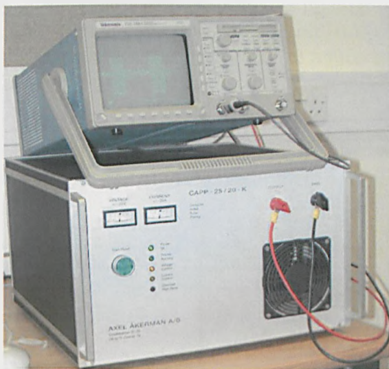
Figure 5.1 The Pulse Rectifier is connected to an oscilloscope displaying a pulse reverse waveform (PR).
