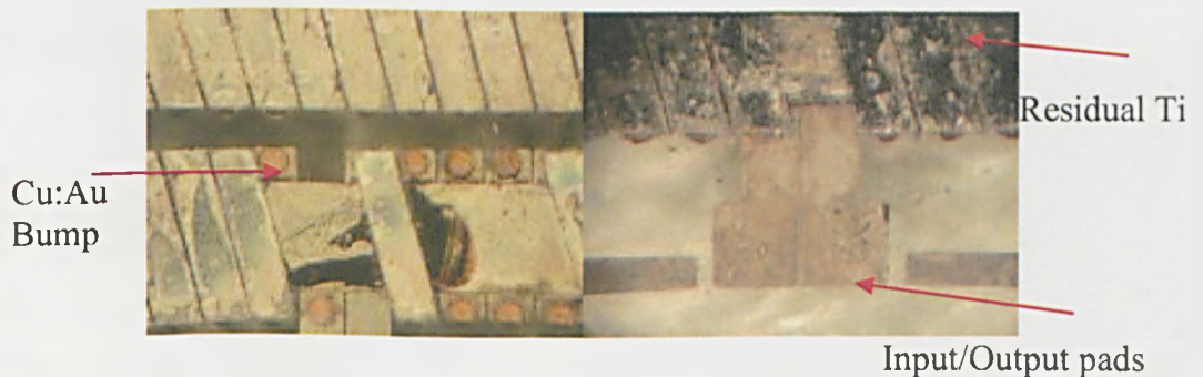
Figure 7.22 Solenoid micro-inductor showing the interconnection between the upper and lower winding layers. The dark material on the nickel is the residual Ti from the adhesion.
