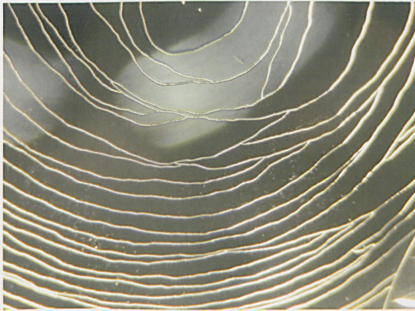
Figure 7.4 Isotropic thermal cracking of a wafer with 10 \mu m thick AZ 9260 layer after the deposition of Ti within the E-beam.
