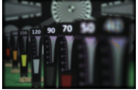
Figure 3: Exemplary refocused photograph. The image has been computed via Eq. (1) using refocusing slice a = 10/9 .
