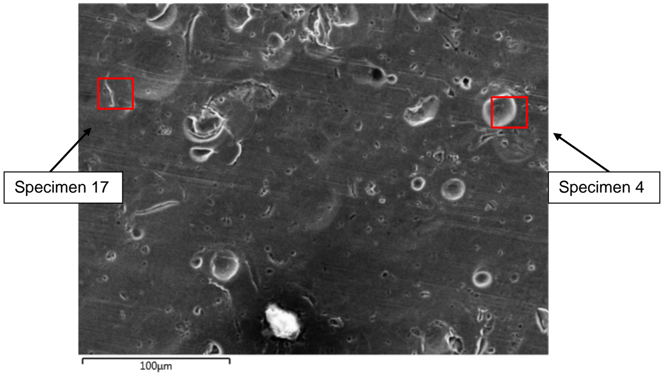
Figure 3-25: X-ray SEM Image of ceramic peened surface prior to friction testing
