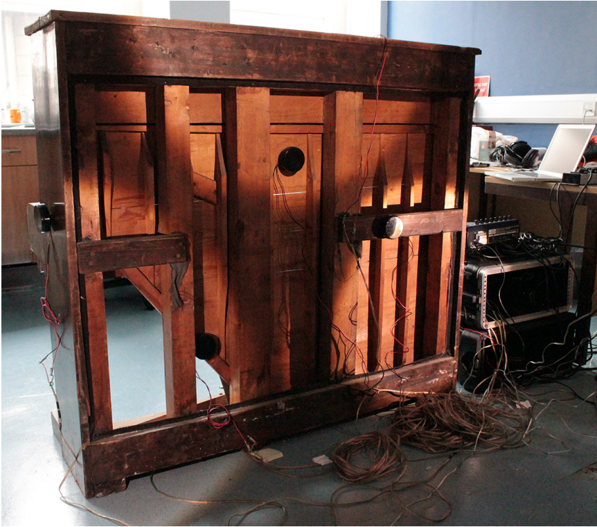
Figure 4.26: The piano equipped with transducers during the development in the ICCMR lab
