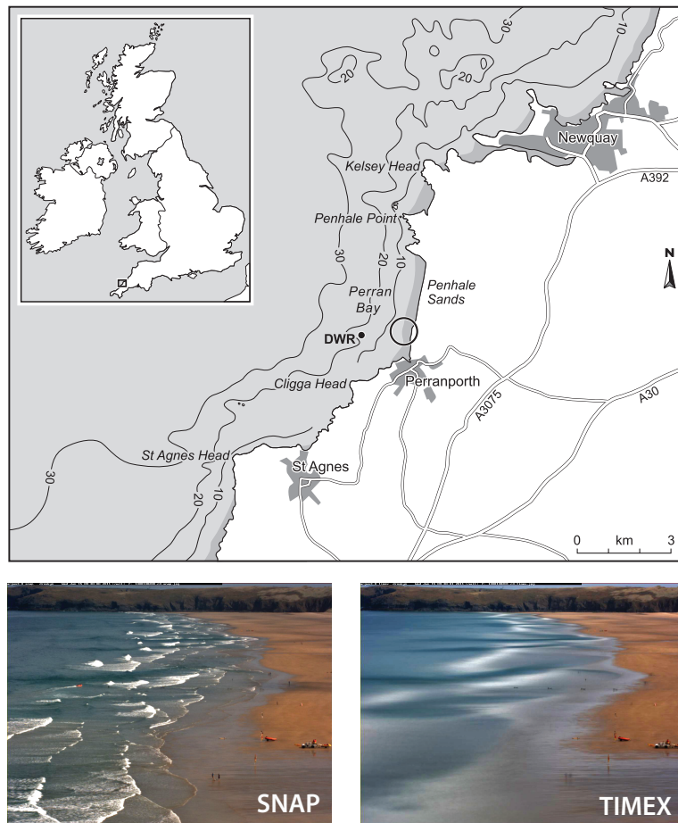
Figure 3: Location map of Perranporth, the site of rip current field experiments during 2011 (upper panel). Study region (circle) and directional wave rider buoy (DWR) are marked. Example Argus video images (snapshot and time-averaged) of rip system during spring 2011 experiment.
