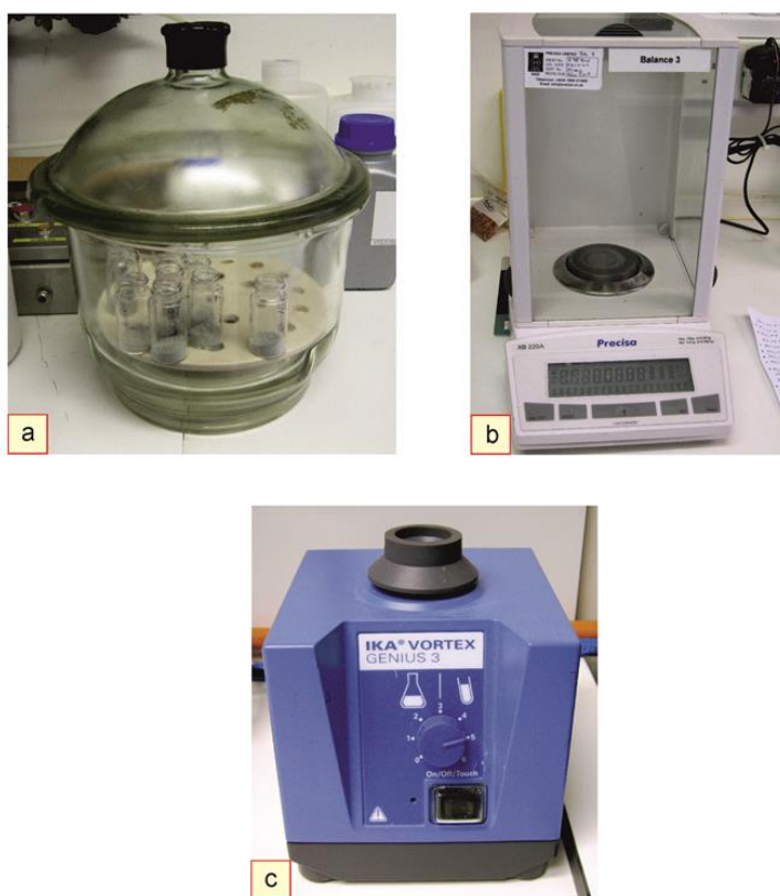
Figure 2.27. Laboratory equipment used for preparing fused beads. (a) Desiccator. (b) Sensitive balance. (c) Mini vibrator.
