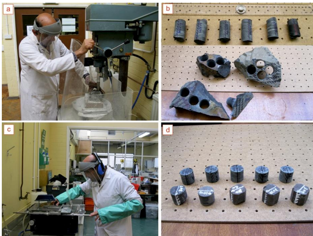
Figure 2.17. Laboratory techniques for preparation of the palaeomagnetic specimens. (a) Drilling the hand samples. (b) Arrows drawn on the side of the drilled cores. (c) Preparing the specimens by cutting the core samples. (d) Numbering the specimens for measuring.
