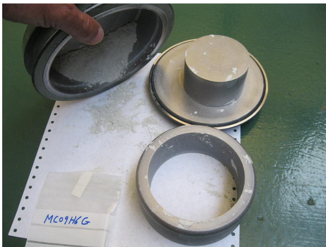
Figure 2.25. Rock powder preparation using the teamer mill.
