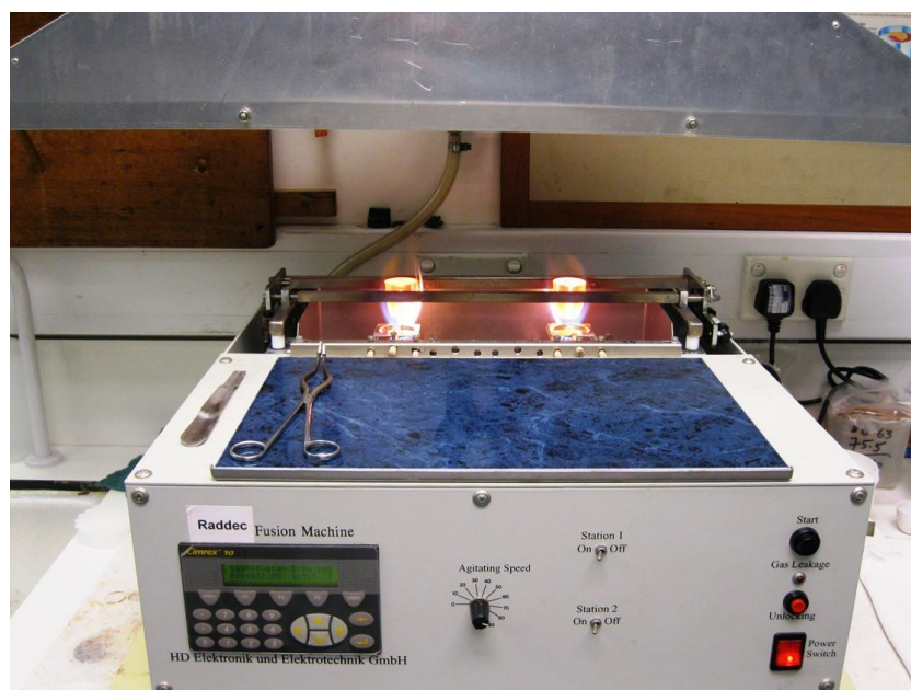
Figure 2.28. Fusion machine used in melting the powder mixtures for preparing fused beads.
