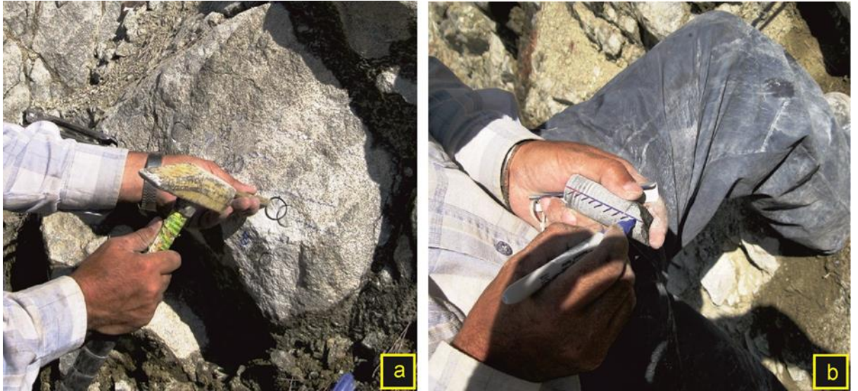
Figure 2.15. Sampling technique used in the field. (a) Collecting drilled samples. (b) In situ marking of a permanent arrow on the upper side of the drilled core in the direction of drilling and labeling the sample with the sample name.
