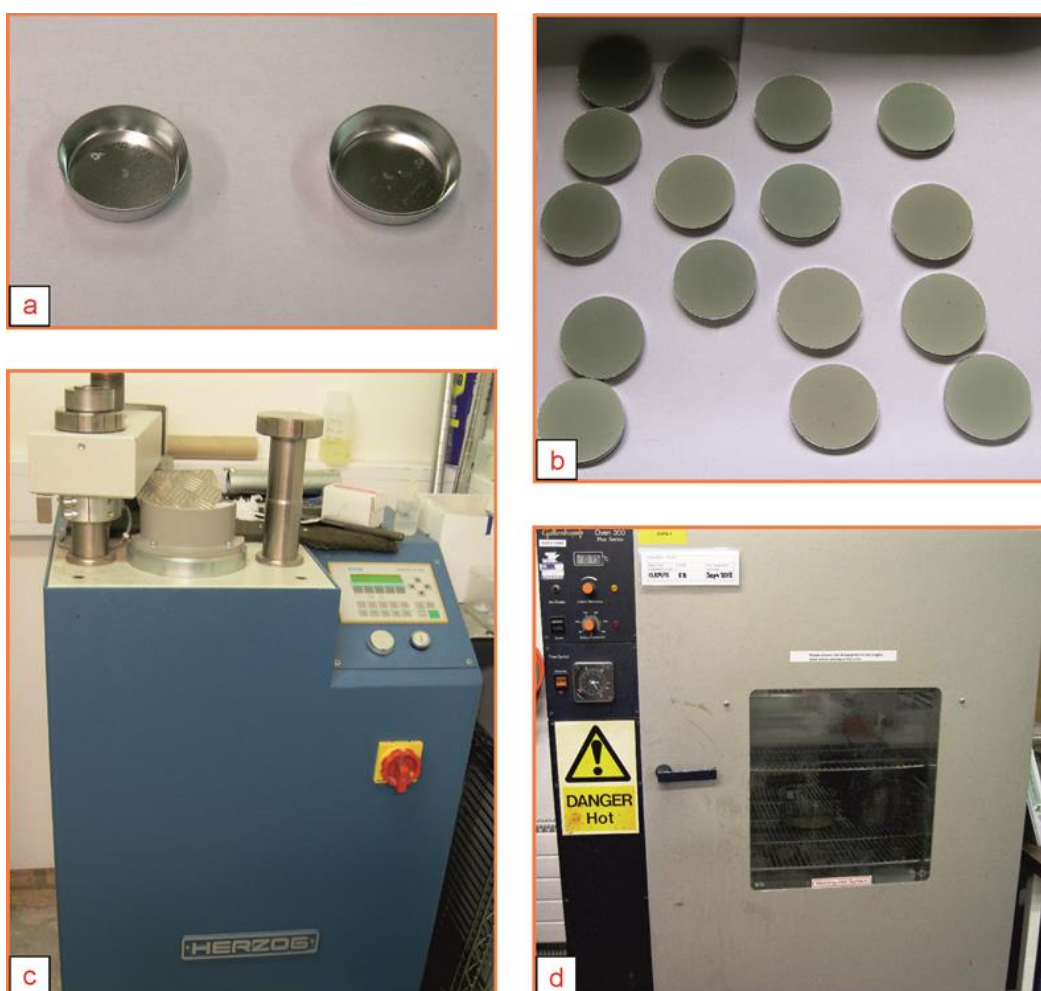
Figure 2.26. Pressed pellet preparation in the laboratory. (a) Aluminum cups. (B) Pressed pellets. (c) Hydraulic press machine. (d) Oven.
