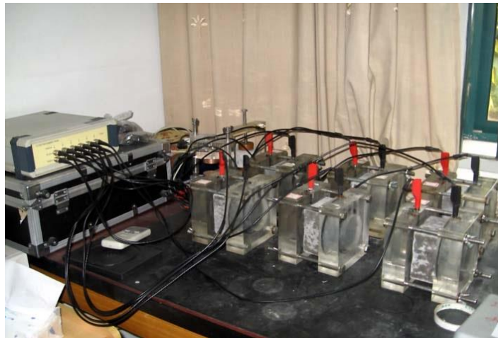
Figure 2.8. Rapid chloride permeability test (AASHTO T277, 1983) set up: schematic (above) and actual (below).
