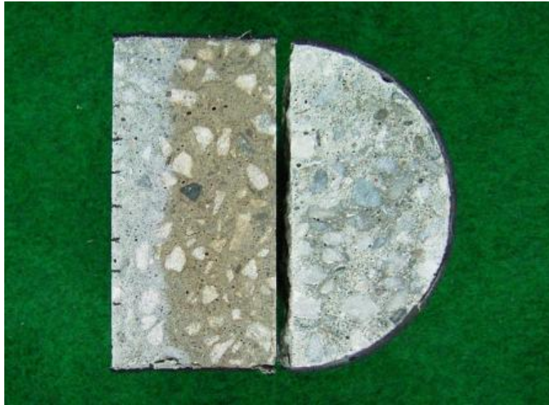
Figure 2.17. Split specimen and penetration depth displayed (Tang and Nilsson, 1992).
