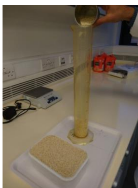
Figure (3.9) Loaf volume measurement
