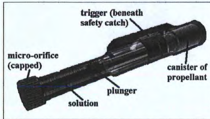
Figure 4-2 Needle-free delivery device: J-TIP® (National Medical Products, Inc.). Reproduced from website[25].
