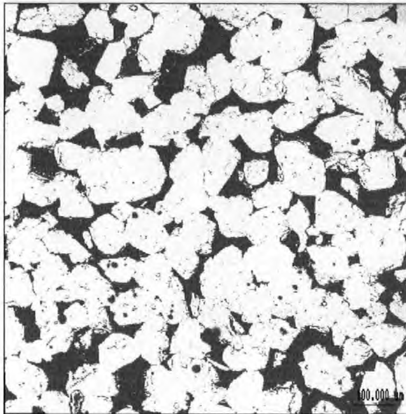
Figure 7.4 Electron micrograph of a resin-impregnated Fontainebleau sandstone sample.
