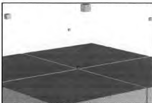
Figure 8.5 A pore configuration that would result in D_4 \ll D_h .
