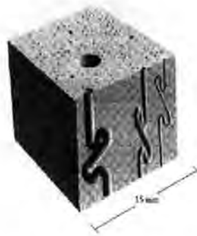
Figure 10.2 Schematic representation of tortuosity
