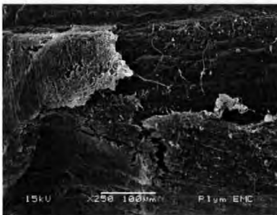
Figure 5.23: SEM image of broken edges of biofilm "coat" seen in Sample B1, replicate Y
