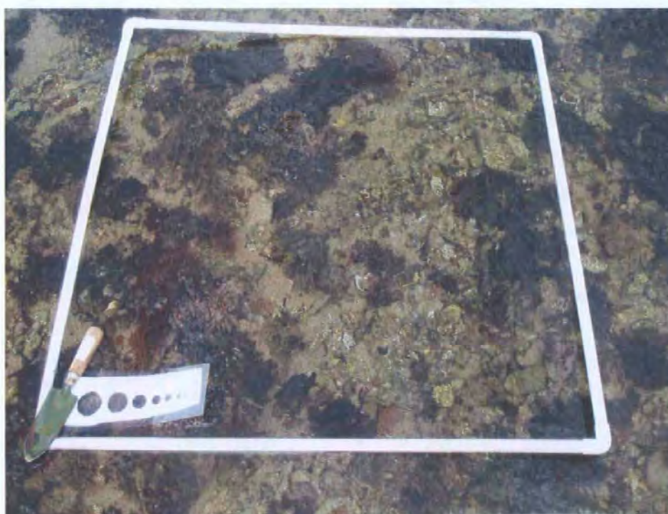
Figure 3.1: Photograph of a study plot at Braunton, showing 1 m 2 buoyant plastic quadrat used to collect sediment size data with the sizing gauge, used to estimate percentage surface area occupied by the different size categories of substrata, visible in the bottom left hand corner.
