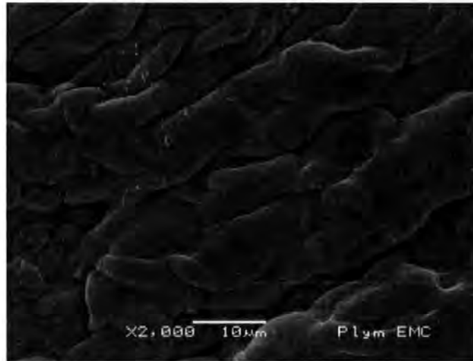
Figure 5.22: SEM image of an area of Sample A2, replicate X, after treatment by brushing/scraping taken at x2000 magnification showing clean surface of thallus
