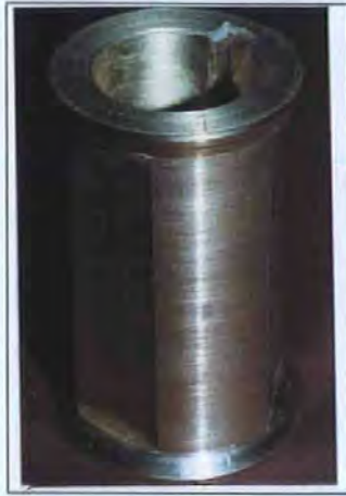
Plate 4.15 HTB1 boss insert in place on a propeller for "Pandora" and the boss prior to moulding.
