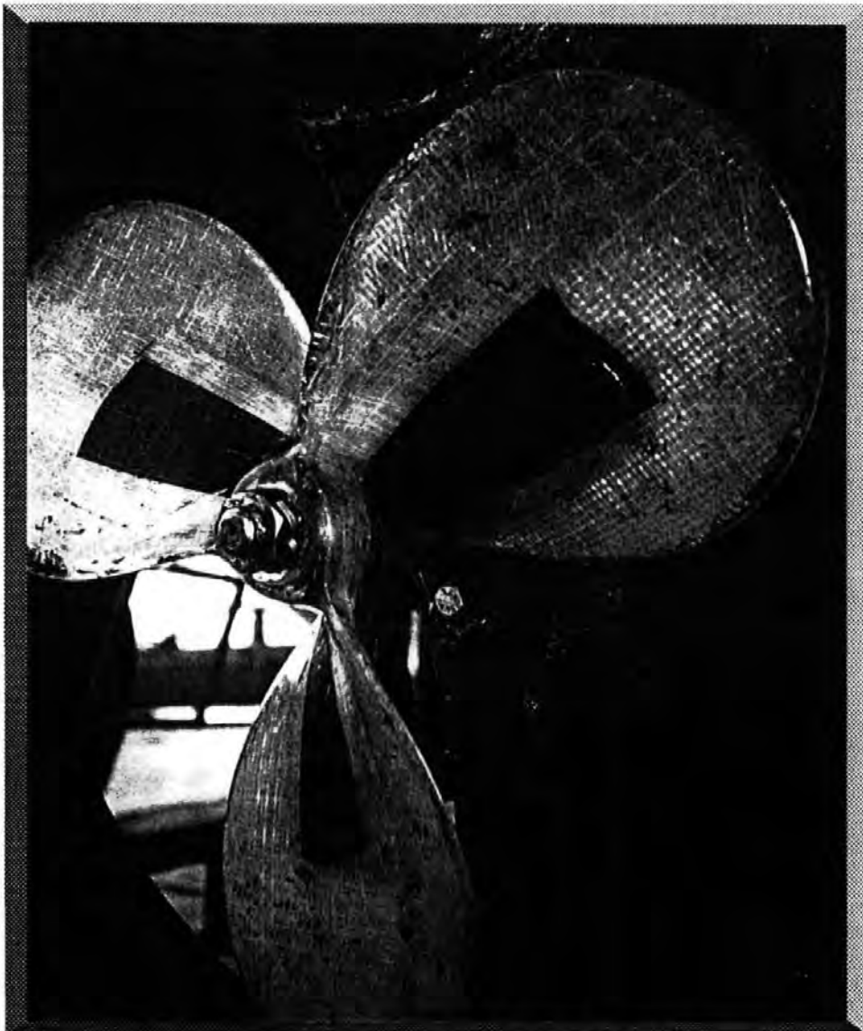
Figure 4. 20 inch diameter composite propeller installed on a 23 foot motor vessel
