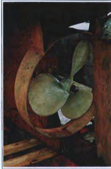
Plate 5.2 The propeller before failure.
