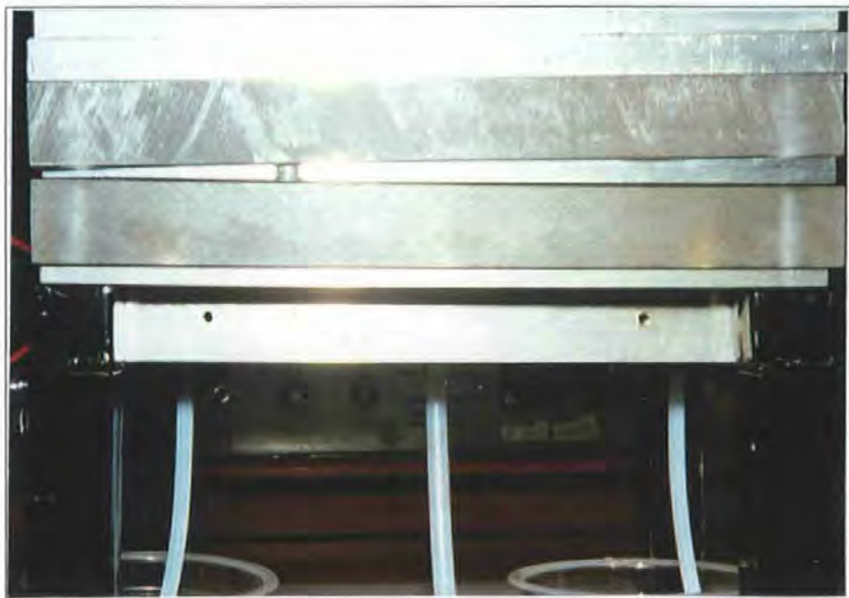
Plate 4.4 Experimental RTM mould (foreground) & Hot Bonder (background) for recording temperature.
