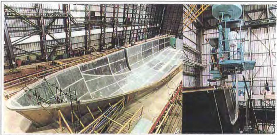
Plate 2.1 Fabrication using pre-wetted glass cloth. (After Anon 1989b).
