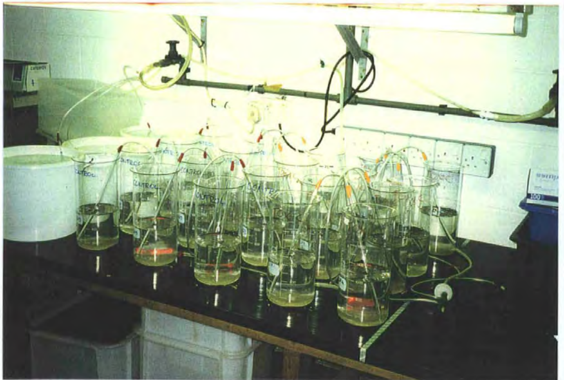
Plate 6.2 (upper plate): addition of exposure water over bubble-wrap to prevent disturbance of consolidated sediment.
