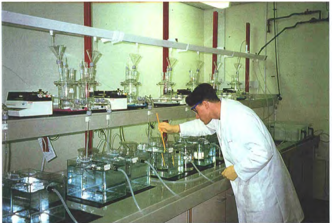
Plate 5.1: The flow-through rig at the Brixham Environmental Laboratory (ZENECA Limited).
