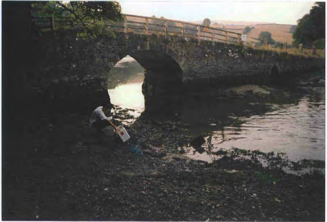
Plate 2.3: Measuring low tide current velocity with the Valeport EM current meter at Terras Bridge, East Looe River Estuary.
