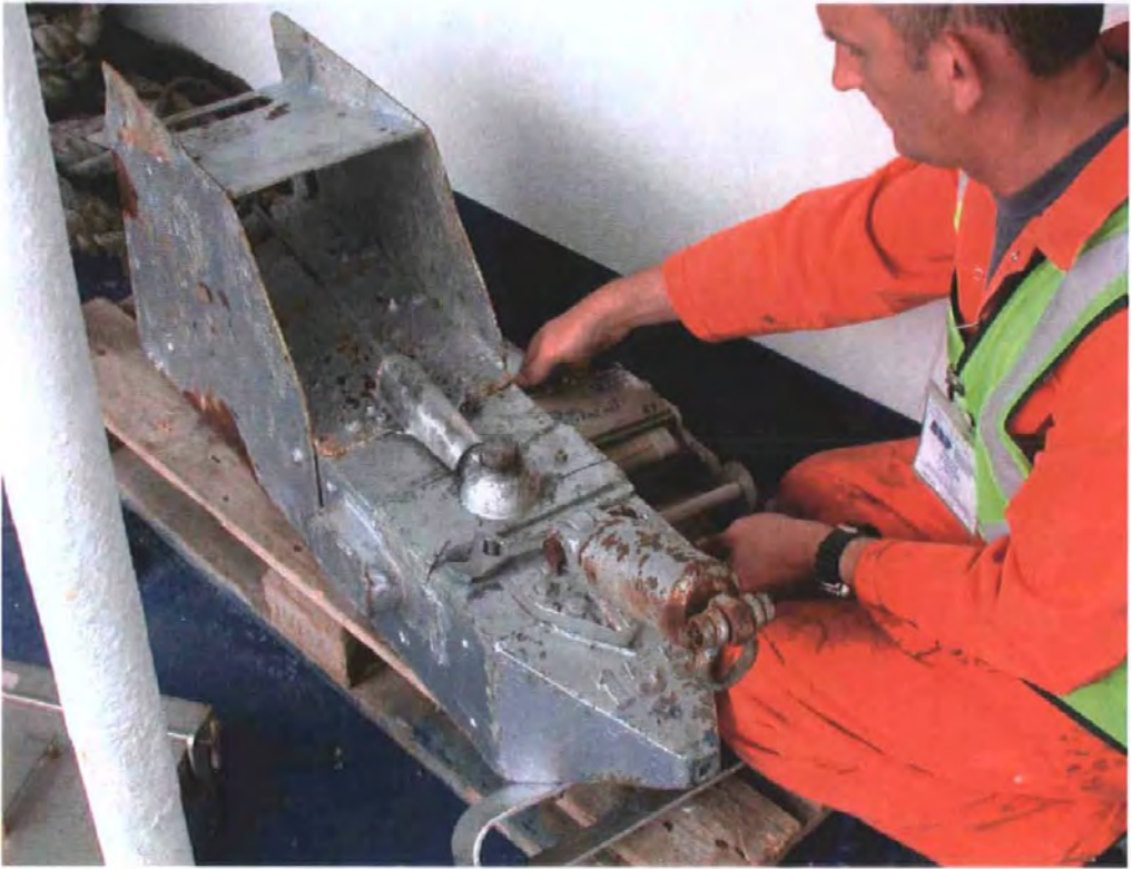
Figure 2.5. Lance Gregory (Marine Technician at SAHFOS) removing the internal mechanism from the CPR body on board a ship of opportunity (from SAHFOS archive).
