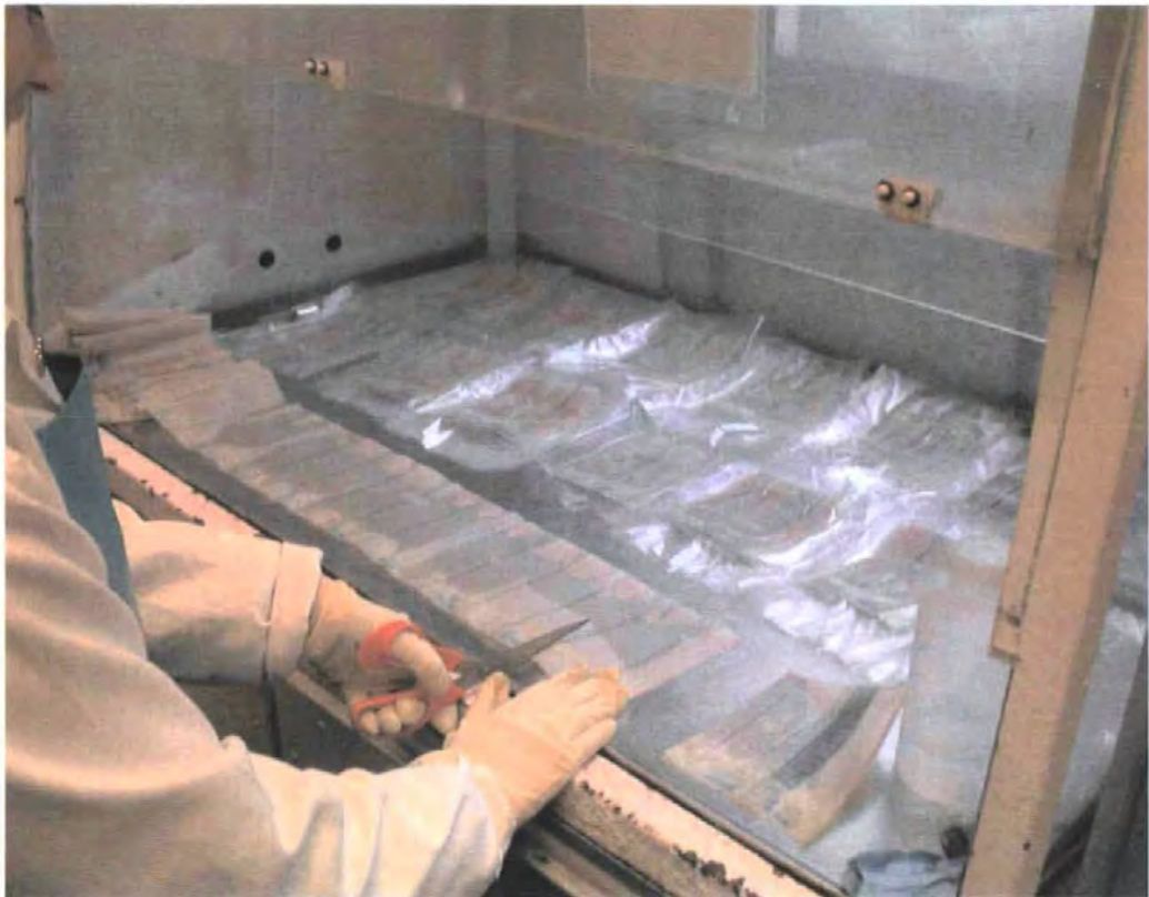
Figure 2.6. The silk is cut into sections (samples), representing 10 nautical miles of tow
