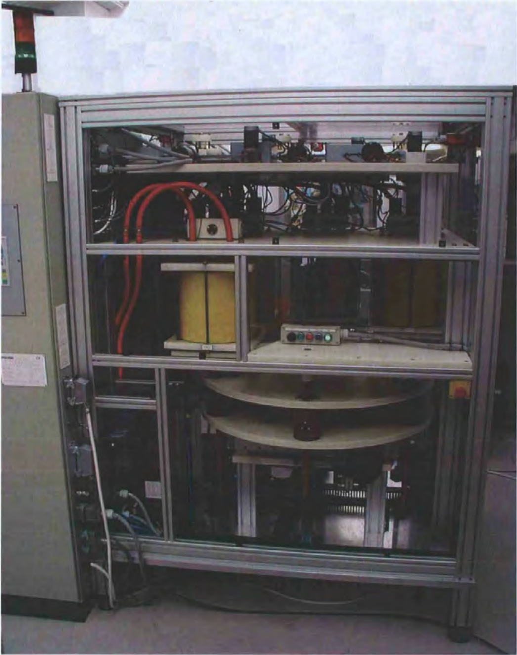
Figure 66 - Completed industrial PFM showing operator station. The (yellow) field generation coils are visible behind the polycarbonate. Magnets are loaded in front of the visible indicator lamps
