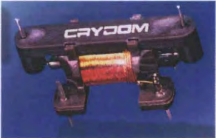
Figure 1.2 – FRS42500 Series (3A @ 30MHz carry current, 3kV isolation)
