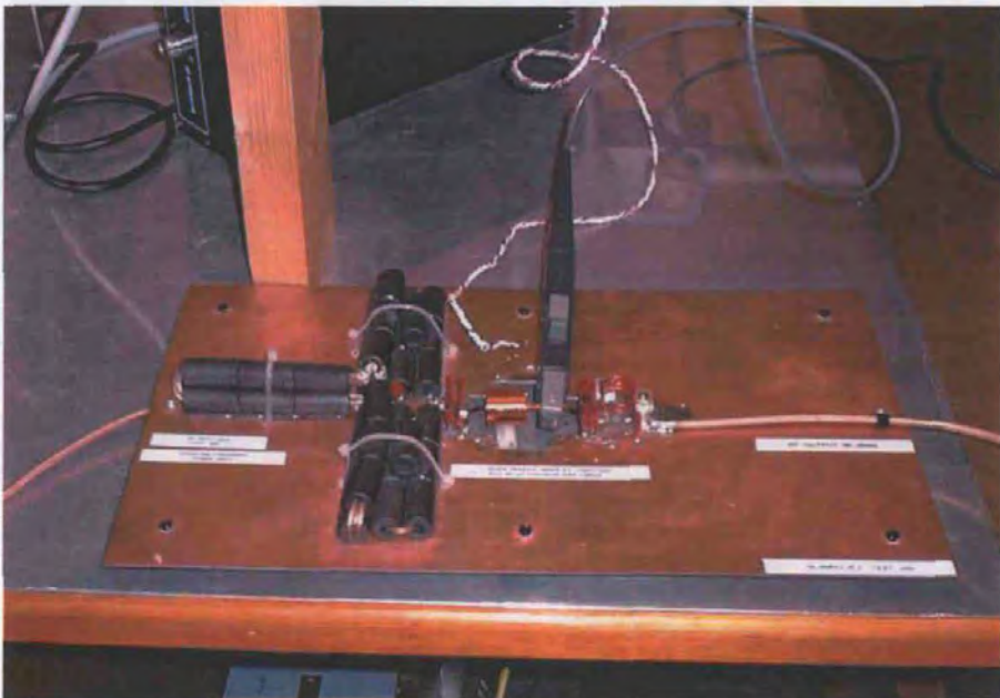
Figure 3.6 – Current Transformer used in High Power Measurements
