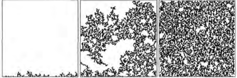
Figure 1: Percolation behaviour on a 2-lattice connected with Moore neighbourhoods ( k = 8 ). From left to right, density \rho = 0.31 , \rho = 0.41 , \rho = 0.51 , respectively.
