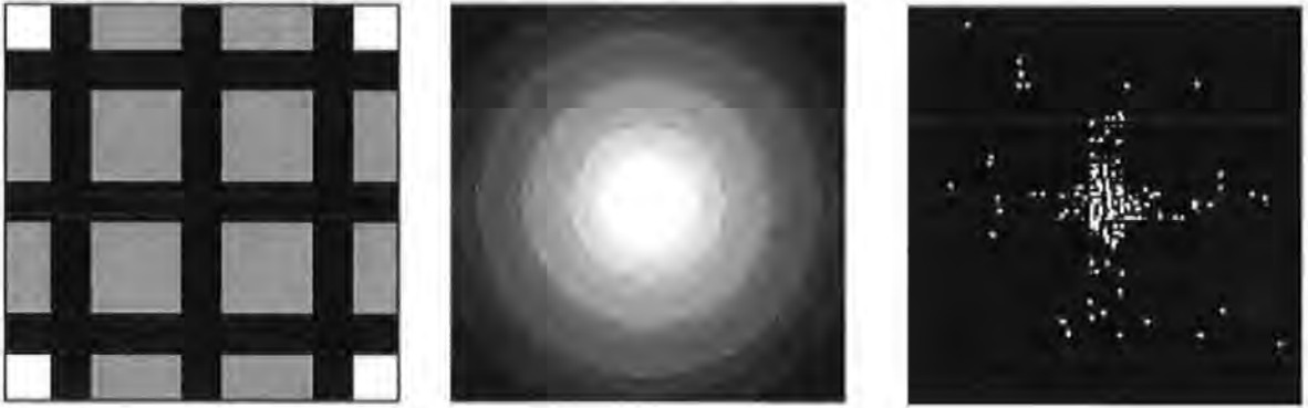
Figure 3.8: A shopping mall model in STREETS. Left: mall configuration. Centre: attraction surface. Right: pedestrian positions after 100 steps. Pedestrian behaviour is determined by a surface of attraction, which is defined globally and without regard for obstacles in the space. Adapted from Batty et al. (1998).
