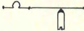
Fig. (11) Schematic diagram of the toggle switch mechanism showing unstable neutral plane position.
