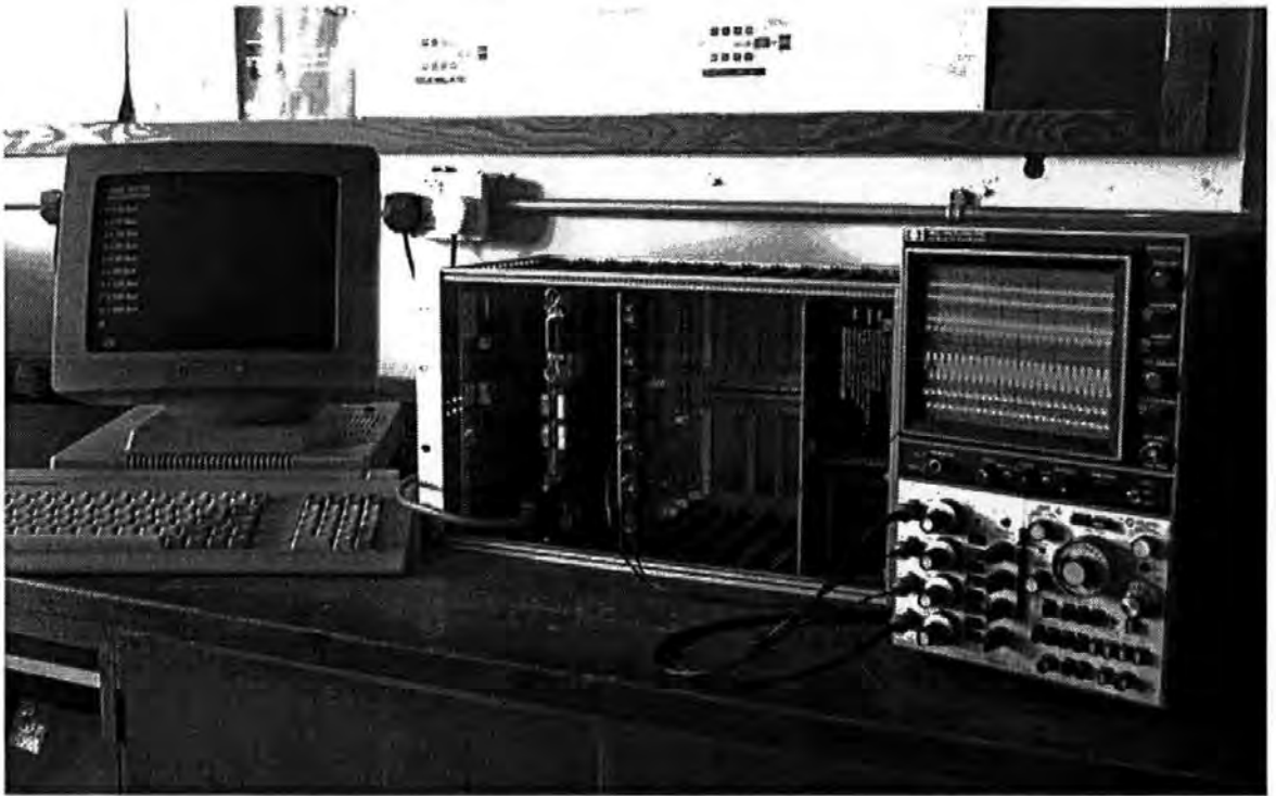
Figure 2-30 Clock recovery test system
