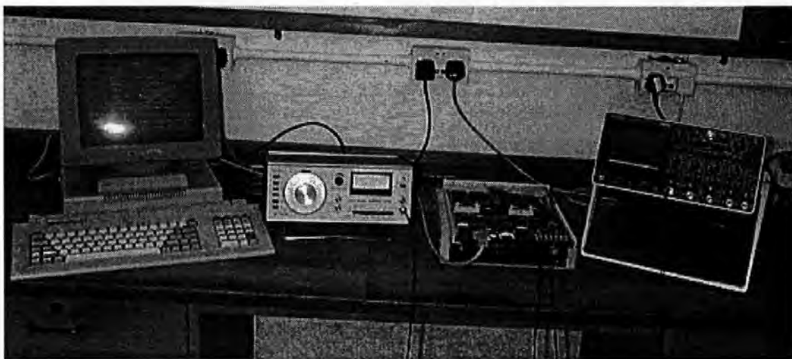
Figure 4-16 Real-time OFFT test system
