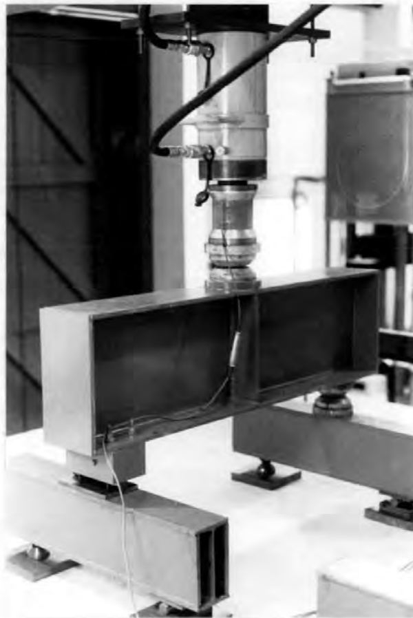
Figure 8.10: Spreader beam assembly
