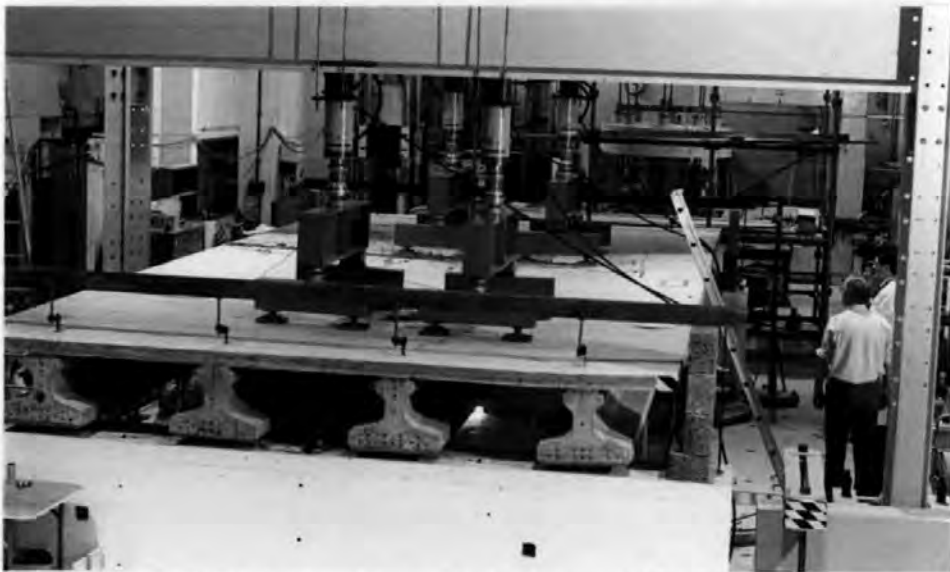
Figure 8.18: First deck under 400kN per jack
