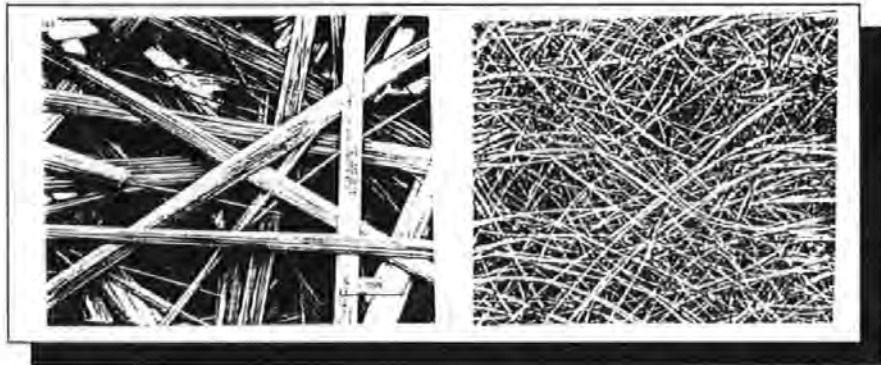
Figure 2:29 Discontinuous (CSM) and Continuous (Unifilo) Random Mat
