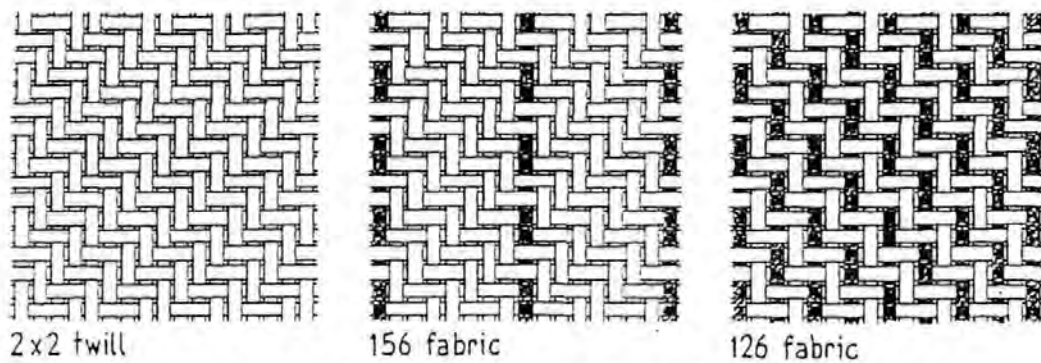
Figure 2 Representative diagrams of the plan view of the reinforcement fabrics. The twisted tows are indicated by shading
