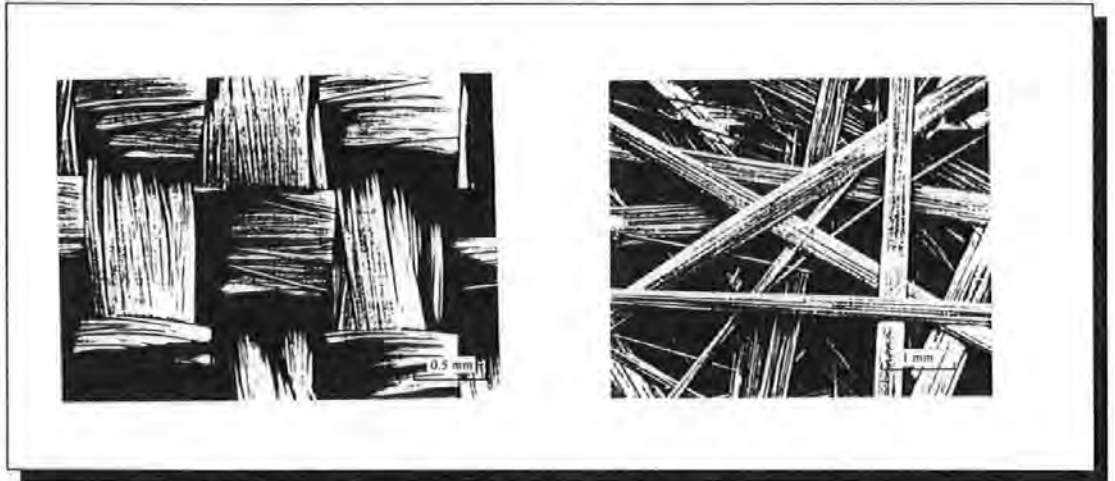
Figure 2:38. A Plan View of a Plain Weave and Chopped Strand Mat (CSM) [5]
