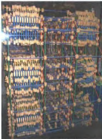
Fig. 134: Danny Hillis' Tinkertoy computer that plays tic-tac-toe, Computer Museum, Boston.
