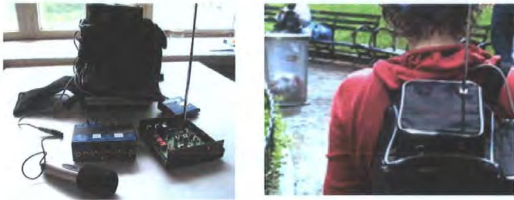
Fig. 16: Com_muni_port is a self-contained backpack transmitter unit used for broadcasting “on the fly.” Its transmission range is determined and limited by the plateaus and canyons of urban space. The dispatch distance updates with movement of its user.
