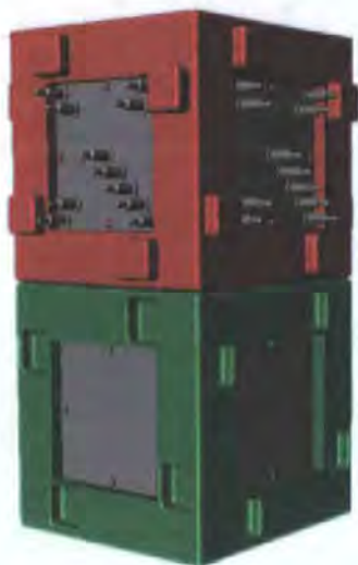
Fig. 61: Stacked male and female appendages CAD model.
