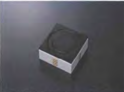
Fig. 153: Single BlockJam block showing connectors.
