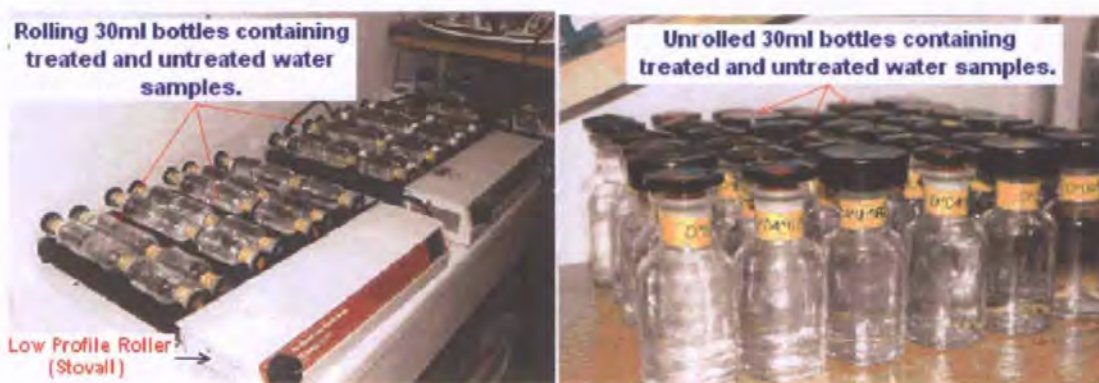
Figure 3.2a-b: Images of (a) the roller system used in the laboratory-facilitated aggregation experiment (Experiments 1 and 2) and (b) benched sample bottles (Unrolled samples; Experiment 1 only) used in comparison with (a) to determine the impact of aggregation on bacterial \text{CH}_3\text{I} production.
