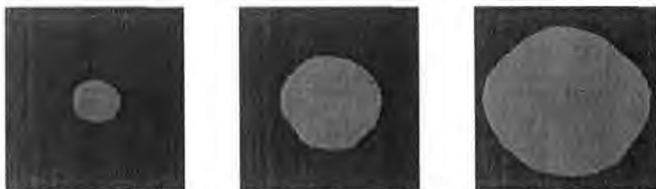
Figure 8: Frame-grabbed images of a typical radial flow permeability experiment at 36, 201 and 653 seconds. The square mould has an edge length of 440 mm.
