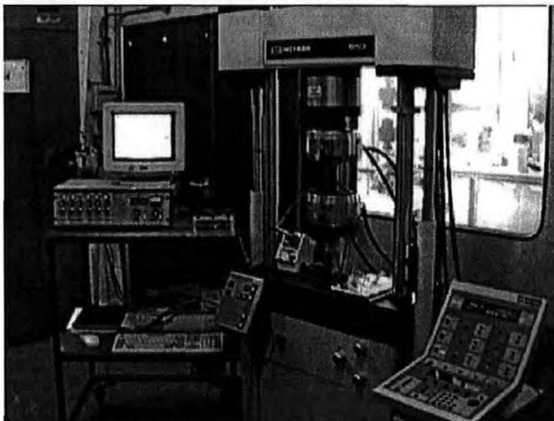
Figure B7-22: Equipment used to test, control and record tension and compression testing
