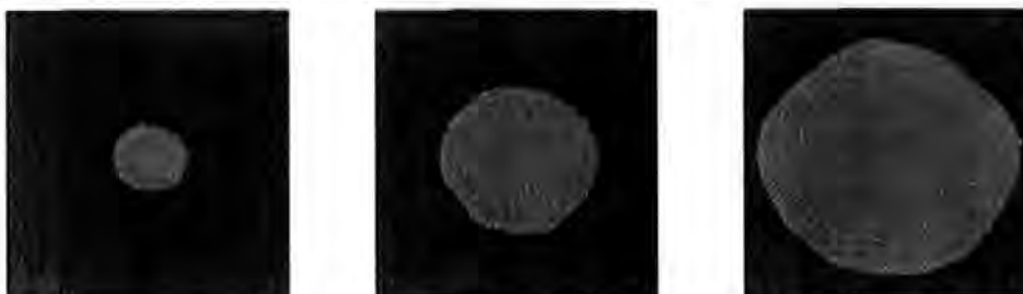
Figure 3: Frame-grabbed images of a typical radial flow permeability experiment at 36, 201 and 653 seconds. The square mould has an edge length of 440 mm.
