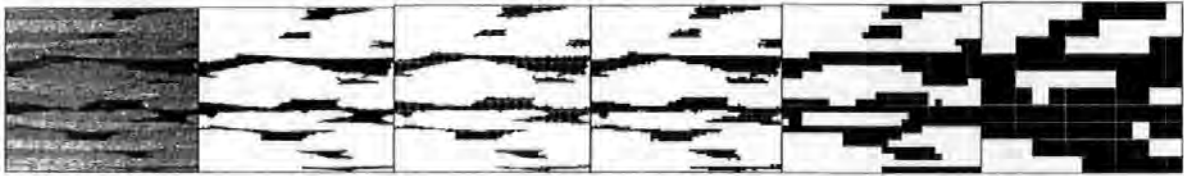
Figure 3: Representative images showing the stages of fractal data generation for a Brochier twill fabric
