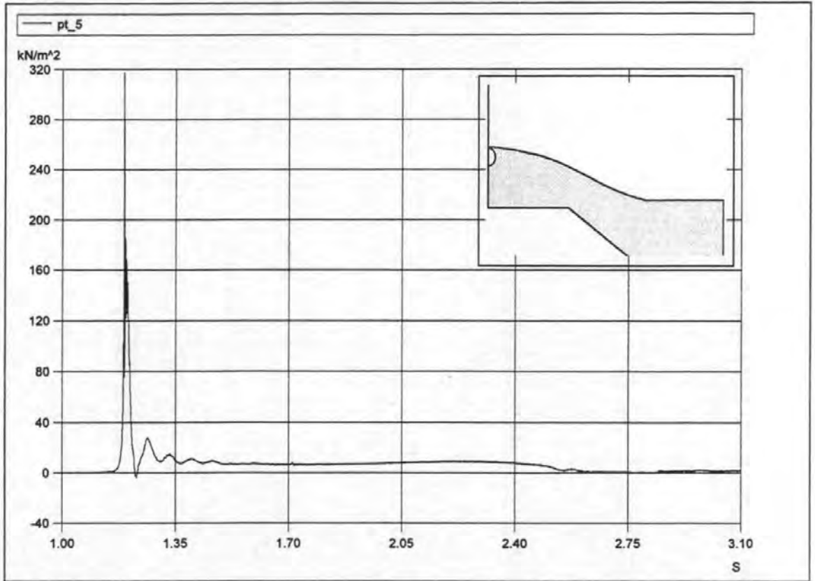
Figure 6.6. Pressure time history of a small air pocket solitary wave impact, H = 0.85 , Test 04029404.
