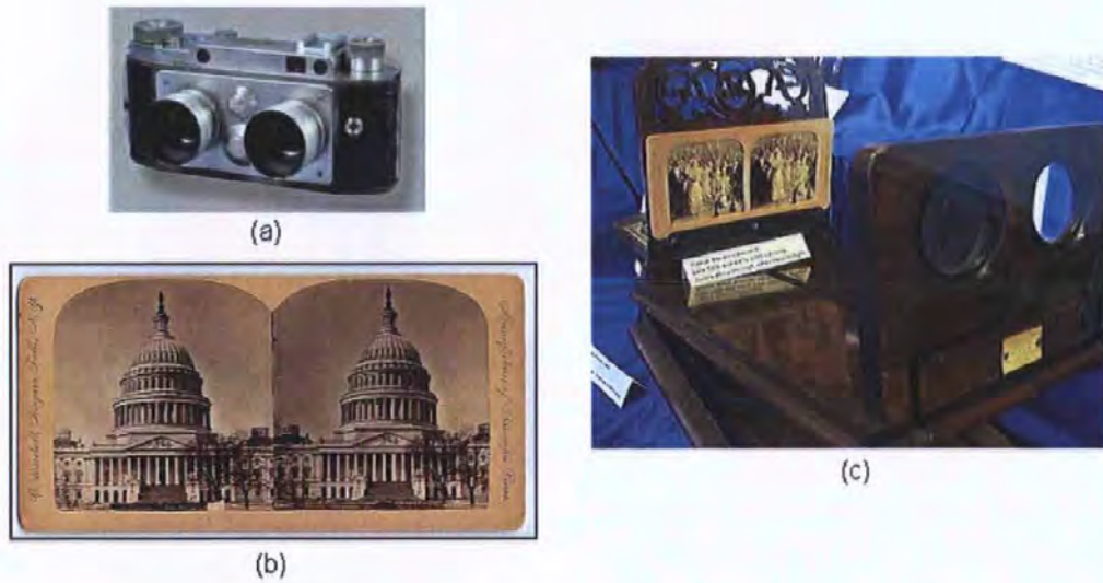
Figure 3.4: Example of 3D photography equipment, (a) a 3D Camera, (b) example photographic image taken with a 3D camera, showing the left and right eye image, (c) a 3D viewer used to present the photographic images to the correct eye
