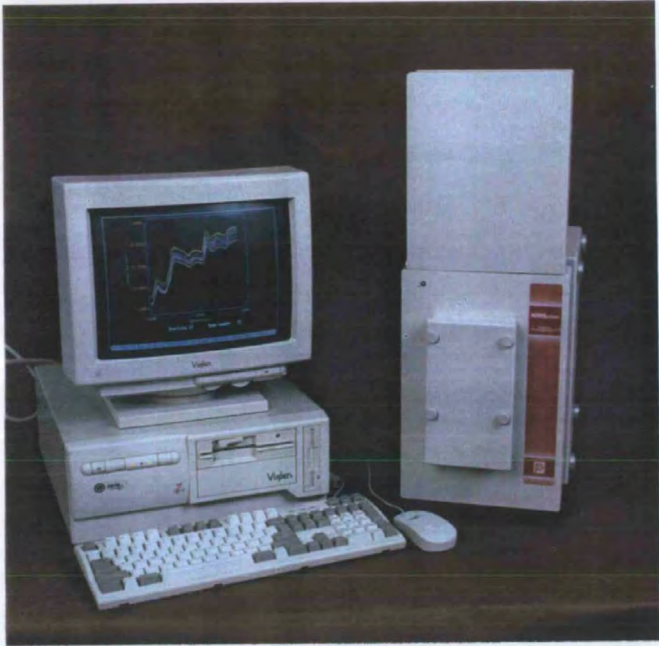
Figure 1.10 An NIRSystems Model 6500 spectrophotometer operating in reflectance and transmittance modes
