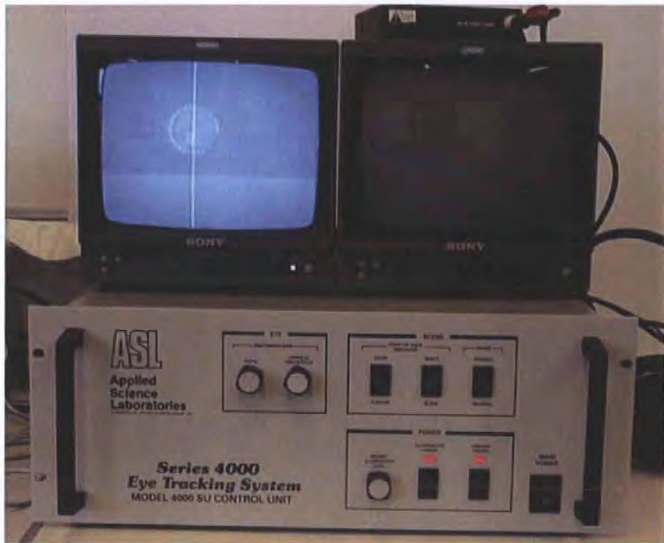
Figure 6.1 The ASL e4000 eye tracker unit. The left screen shows two crosshairs – the first locates the centre of the retina and the second shows the location of the corneal reflection.
