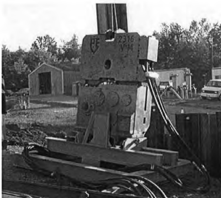
Figure 9. A PVE 2316 VM vibropiling driver. It is shown resting in a cradle made of I-section beams.
