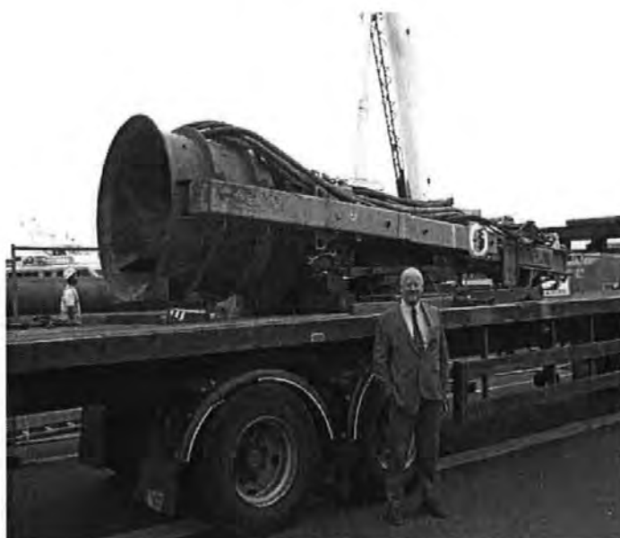
Figure 10. A view of the lower end of the BSP 357/9 Hydraulic Drop Hammer used for impact driving, while it was lying on a lorry.
