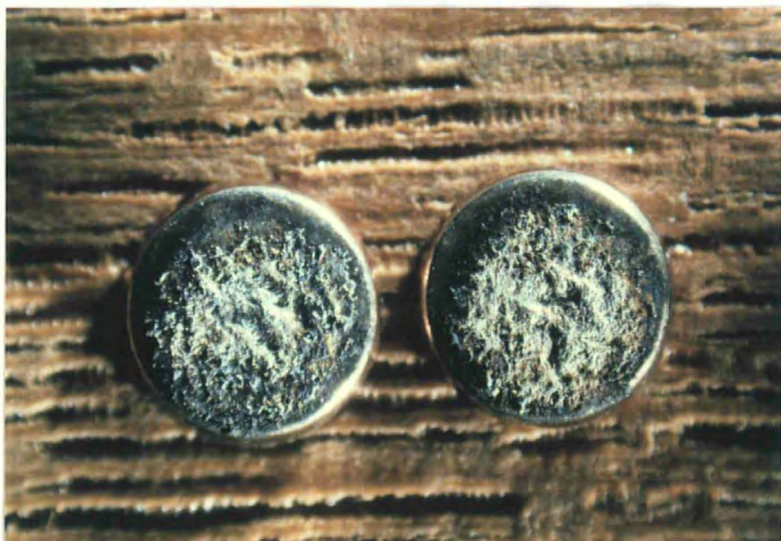
Figure 5.23 The eroded contacts used for the data in figure 5.22, after 10,000 operations at 16 Amps a.c
