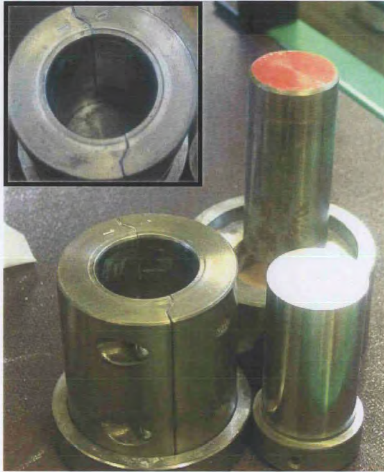
Fig. 43 The present die design. In front left the die with improved dividing mechanism, front right the piston, behind it the template as an option to push the formed tablet out by the press. Little image top left, top-view of the improved dividing slit.
