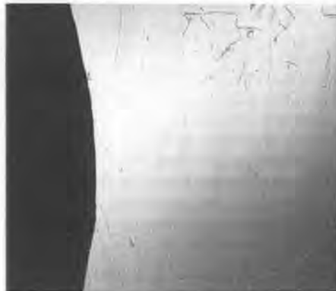
Fig. 19 Equilibrium edge of a drop of glycerol (dark image) on a naturally smooth surface of calcite. More details see Fig. 20.
