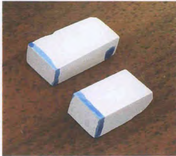
Fig. 98 Samples for imbibition: cuboid blocks of compressed porous structures with wax barrier around basal edges to prevent surface wicking.
