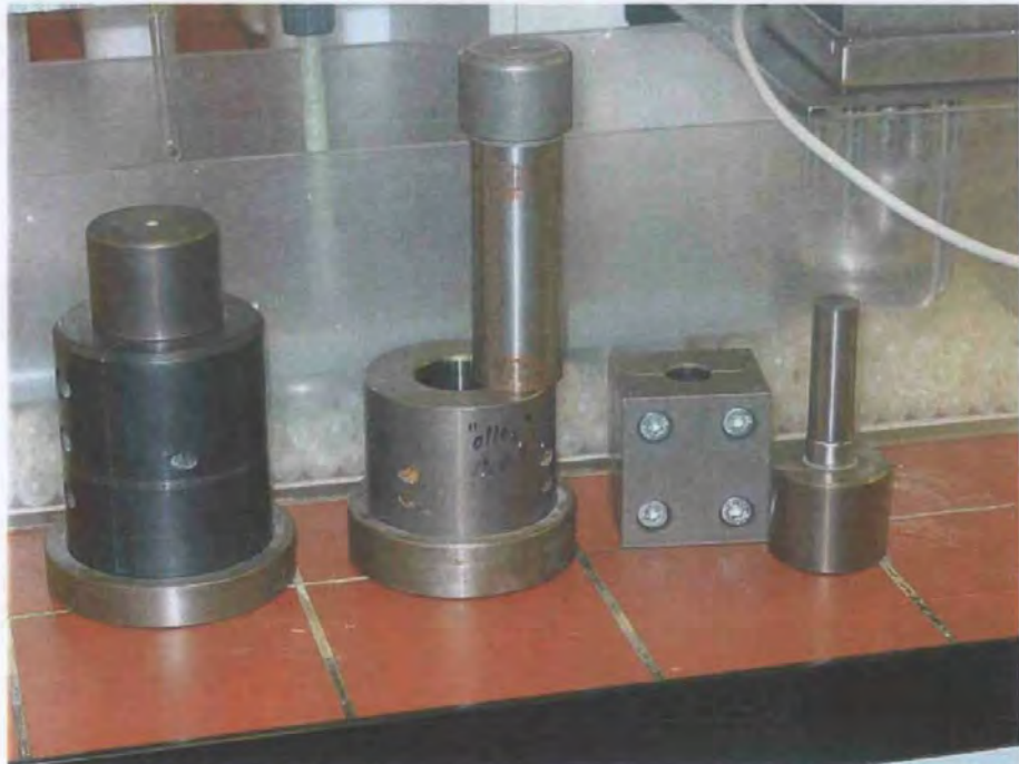
Fig. 42 Development of dies from left to right. (i) The first prototype, found to be too heavy and steel quality too soft, the design also omitted any end-buttet screws to help push the two sections apart. (ii) Improved lighter version but wore out after the production of \approx 200 tablets. (iii) Die with a smaller piston diameter to achieve higher pressures, dimensions did not withstand the high pressure and deformed.
