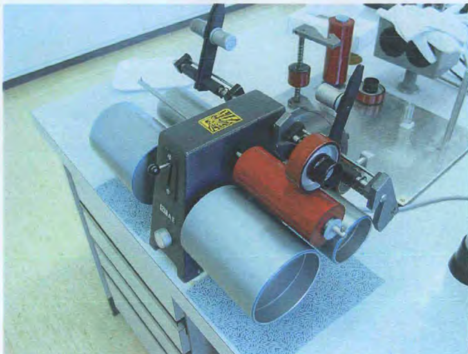
Fig. 36 IGT Inking unit, shown without applied ink. On the right hand side the rubber distribution rolls are in place and the print wheel is on top.
