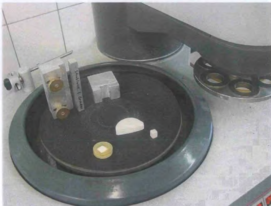
Fig. 46 Automated grinding machine (Jean Wirtz, Phoenix 4000). On the disc at the back are the custom-made grinding jigs. Front left: sample embedded in resin for permeability measurement, middle: half of a pigment tablet, right: sample ground to finished dimensions ready for the imbibition experiment.
