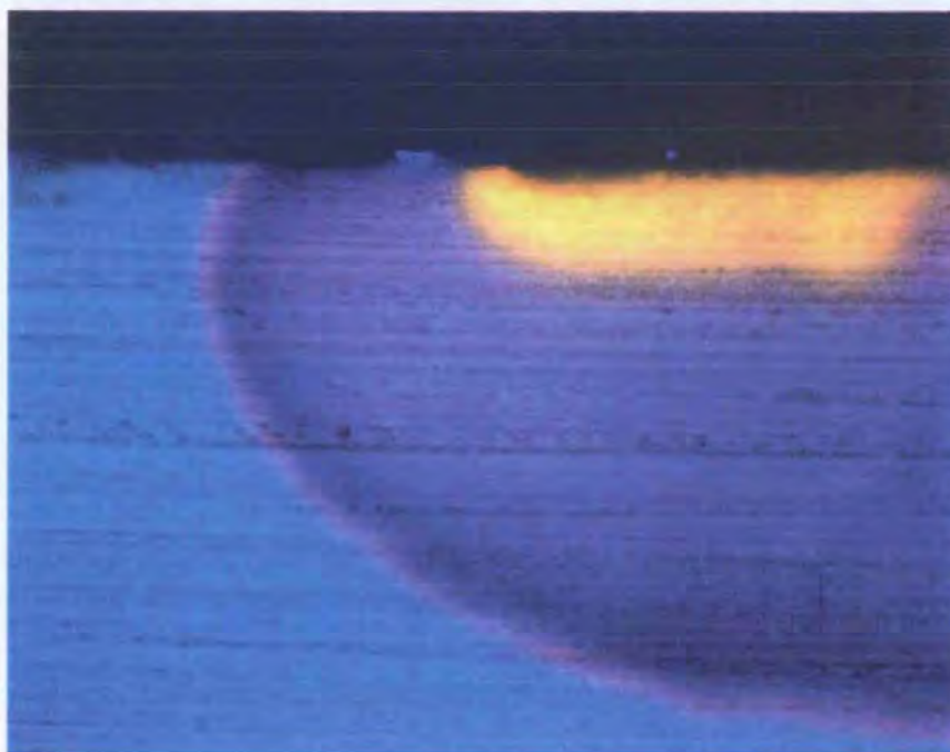
Fig. 68 The picture displays the cross-section view under the fluorescence microscope of the dyed tablet space after imbibition of a blend of equal amounts of Rhodamine B (orange, retarded) and Aluminiumphthalocyanine-sodiumsulphonate (dark blue, advanced). This shows impressively the chromatographic effect. (Magnification 50x).
