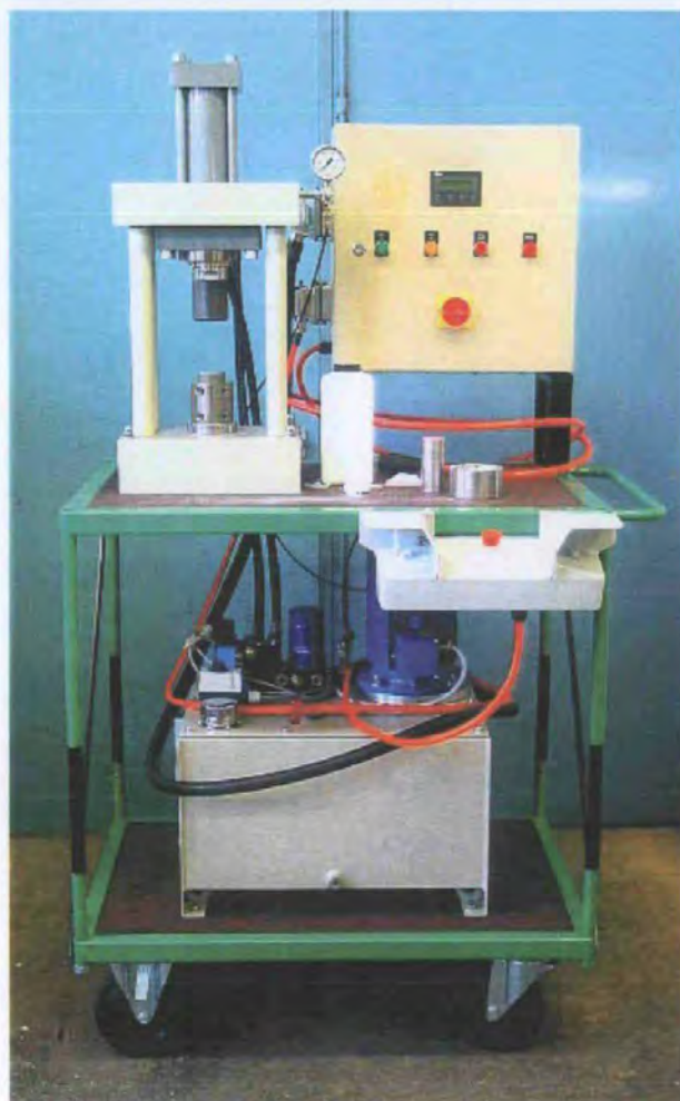
Fig. 44 Custom-made hydraulic press for tablet compaction. On the bottom is shown the hydraulic unit, top right the electronic steering unit and the press-frame with the hydraulic cylinder exerting a force up to 600 kN.
